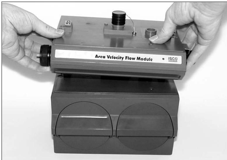
*Figure 1-21 Aligning the modules*
