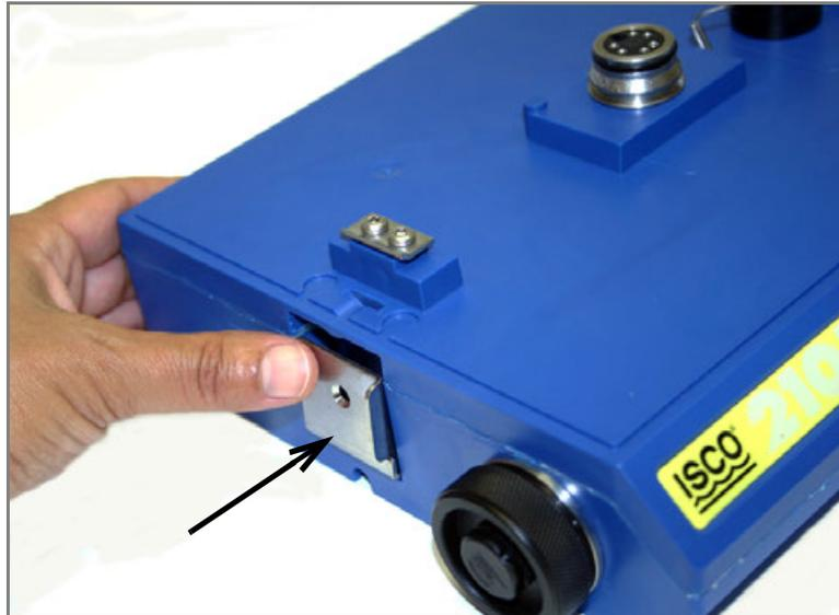
Figure 2-4 Locking the latch
