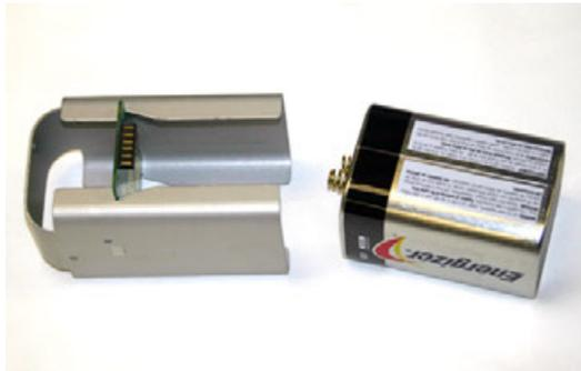
1. Load the lantern battery into the carrier.
