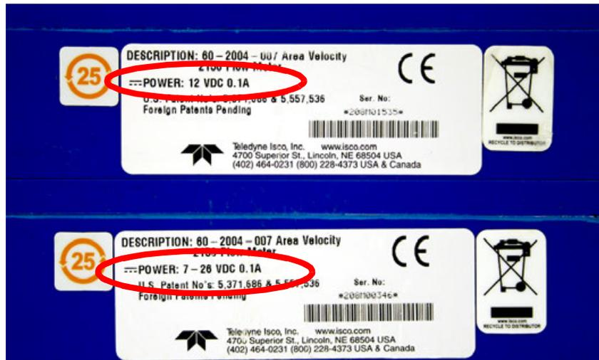
Figure 2-1 Identifying the 2150 voltage specification
