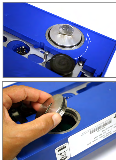
Figure 3-2 Accessing the SIM card on the bottom of the module
