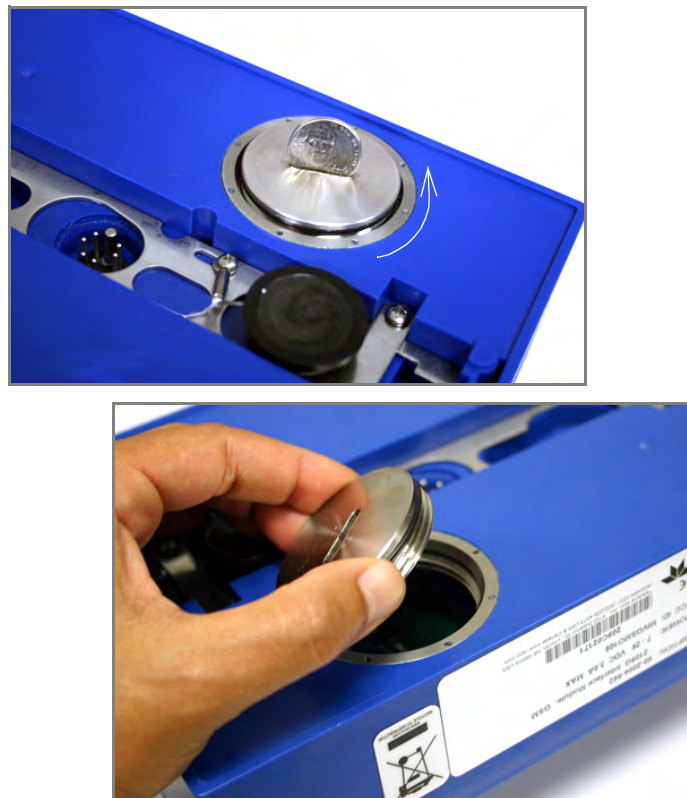
Figure 4-2 Accessing the SIM card on the bottom of the module
