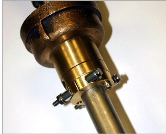
*Figure 2-48 Early version Hot Tap with secondary collar installed*
