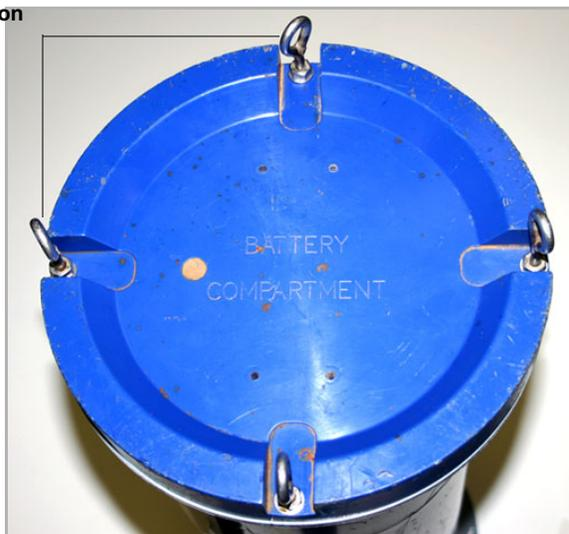
Figure 2-59 Canister: remove battery compartment lid
