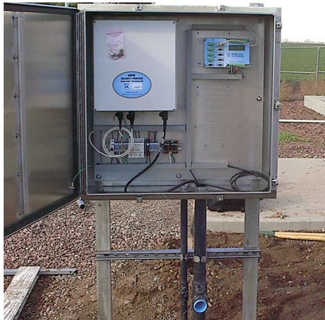
*Figure 2-20 ADFM controller: environmental console enclosure*
