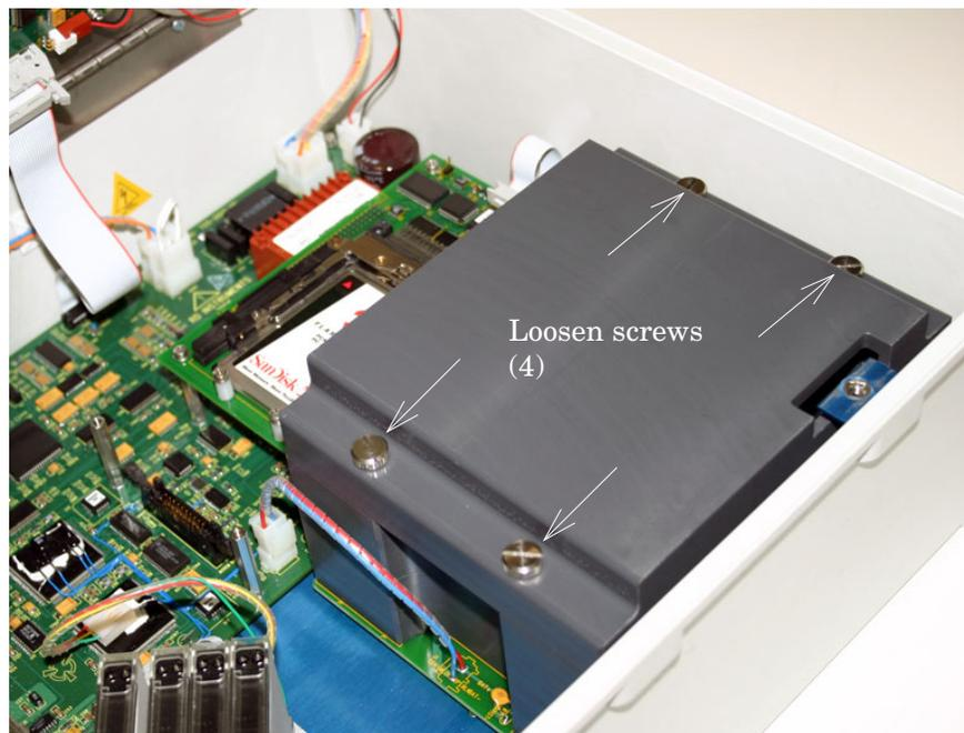
*Figure 2-55 Box controller: remove the battery compartment*
