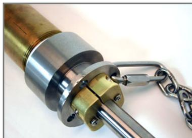
Figure 2-52 Attaching the tether chain
