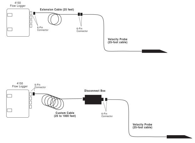
Figure 2-15 Cable Connections and the Quick Disconnect Box
