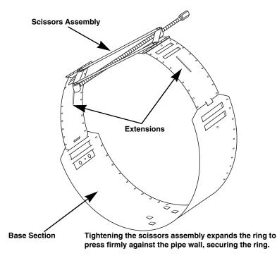
Figure 2-7 Scissors Ring Adjustment
