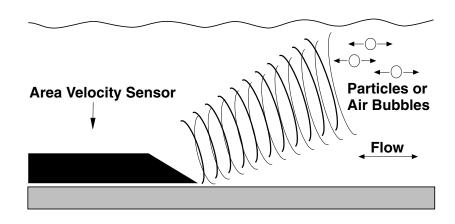
Figure 2-3 Area Velocity sensor Operation
