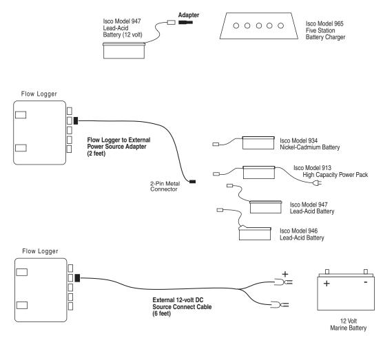
Figure 2-13 Adapters for Alternative Power Sources
