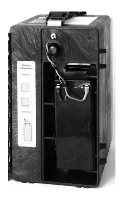
Figure 2-8 Installing the 947 Lead-Acid Battery
