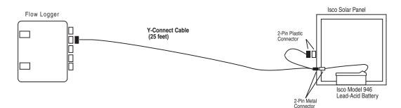
Figure 2-10 Connecting Solar Panels to the 4150
