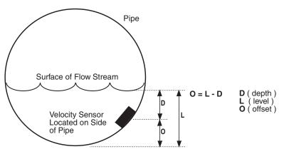
Figure 2-4 Calibration Measurements
