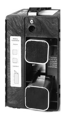
Figure 2-9 Installing Alkaline Batteries
