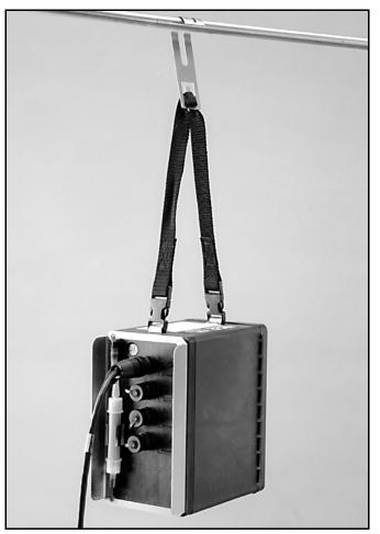
Figure 2-2 Suspending the 4150 (suspension handles may vary)
