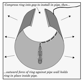
Figure 2-6 Sensor Installed on a Spring Ring
