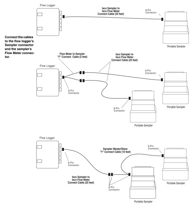
Figure 2-14 Connecting Samplers to the 4150
