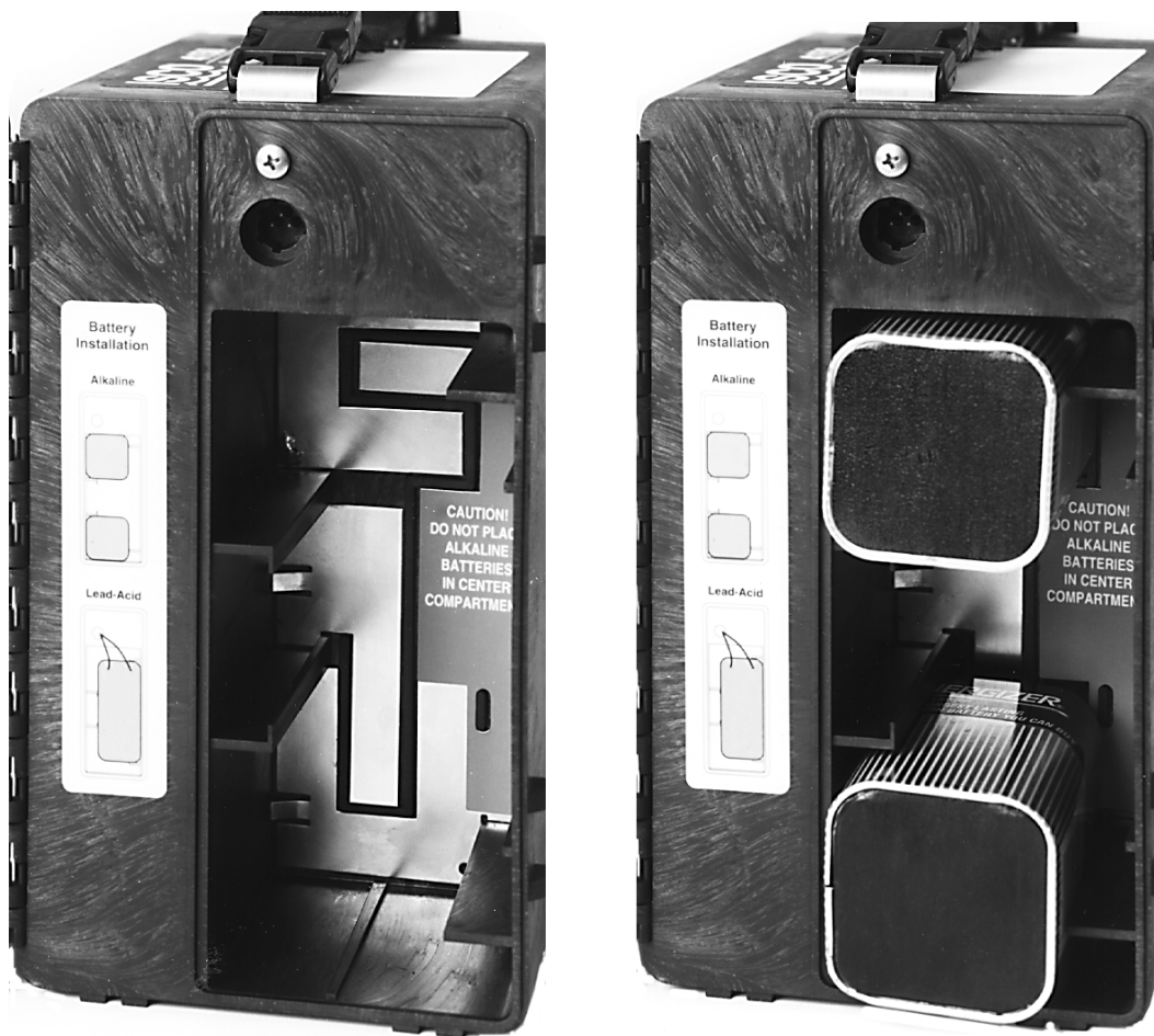
Figure 4-4 Installing Alkaline Batteries
