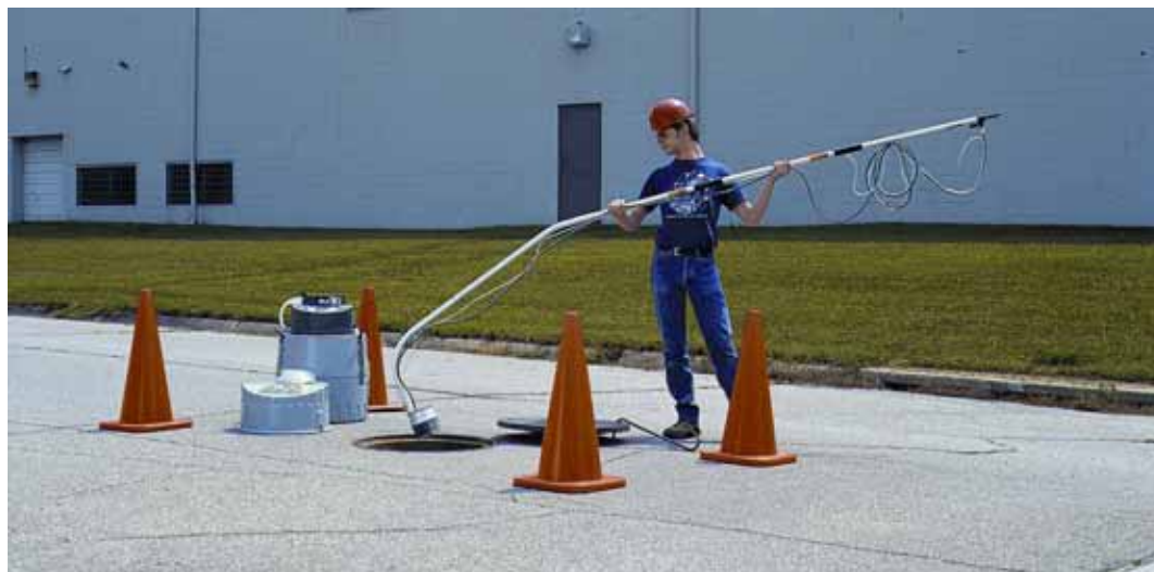
Flow Metering Inserts eliminate the costs and hazards of manhole entry and the need for weirs or flumes.
