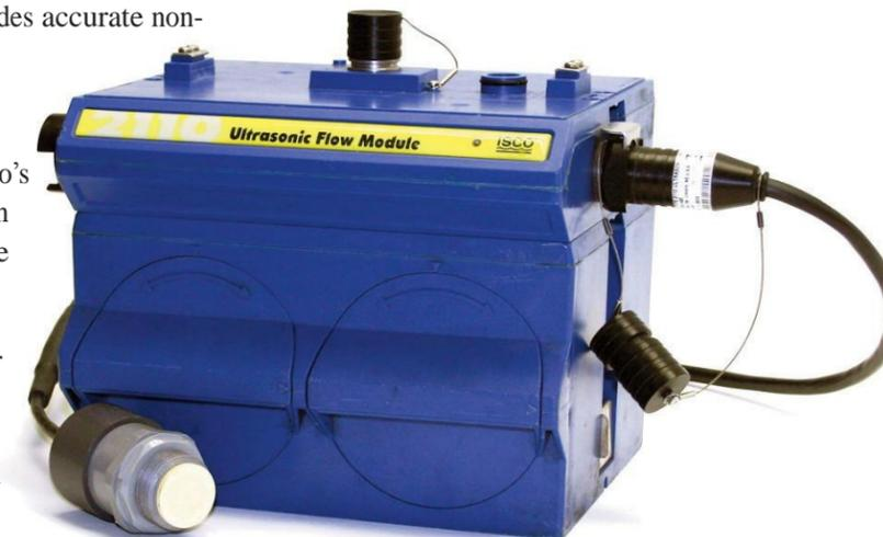
With the 2110, an ultrasonic sensor mounted above the flow stream transmits sound waves, which are reflected by the liquid surface. The elapsed time between transmitted and returned signals determines the liquid level.
