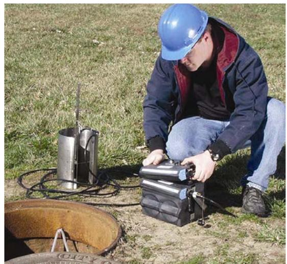
The 2150EX is approved to the ATEX Directive 94/9/EC by Baseefa, and to Class I, Division 1 by CSA for use in manholes and other hazardous locations. A second flow module can be stacked to provide redundant or multi-stream measurement.
