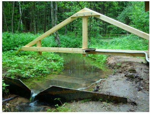
Typical stream monitoring application with V-shaped weir, ultrasonic level sensor and automatic water sampler.
