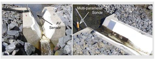
Monitoring Site with 2150 AV Sensor in Trapezoidal Flume and Multi-Parameter Sonde
