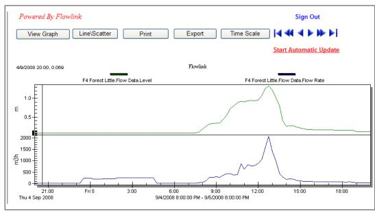
Flowlink WebUI: The web page above displays storm event data from an installation site where the flume's max level was surpassed, but flow was still measured using area-velocity rather than a level-to-flow calculation.
