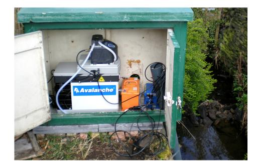
A typical remote CSO monitoring station with a Teledyne Isco Avalanche refrigerated sampler, multiparameter sonde, and 2105G interface module.
