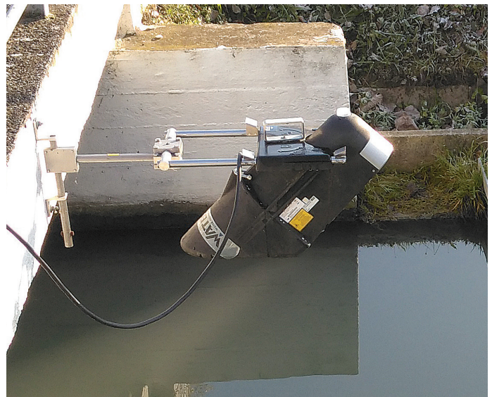
LaserFlow sensor attached to the bridge
