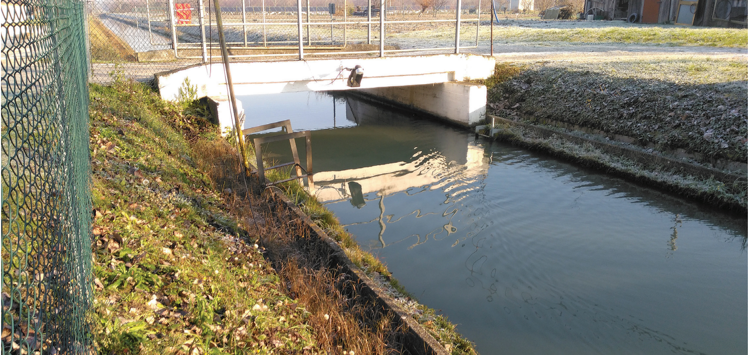
LaserFlow sensor installed over 4 m wide channel upstream the inlet of WTW.
