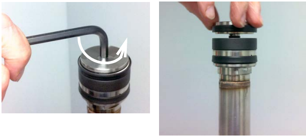
Figure 7: Separate retainer from piston
