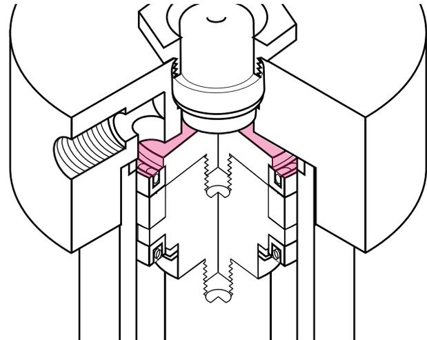
**Figure 3: Dead volume remaining at top of stroke (shaded area)**
