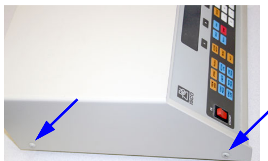
Figure 3: Controller case top screws (2 of 4 shown)
