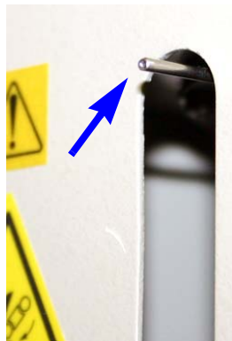
Figure 2: Close-up of nitrogen purge tube
