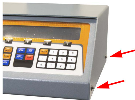
Figure 9-5 Controller case top screws (2 of 4 shown) - TBD
