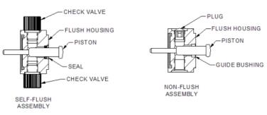
Figure 1-2 Self-flush and non-flush assemblies
