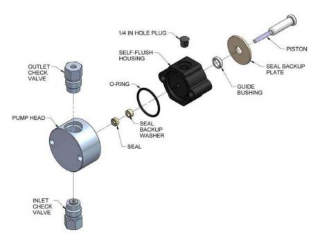
Figure 5-4 Stainless steel non-self-flushing pump head assembly
