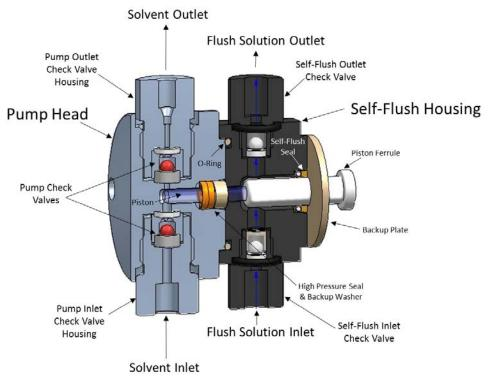
Figure 1-1 ReaXus self-flushing pump head
