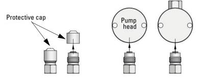
Figure 5-6 New check values from package in proper orientation
