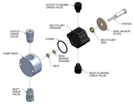
Figure 5-3 Stainless steel self-flushing pump head assembly
