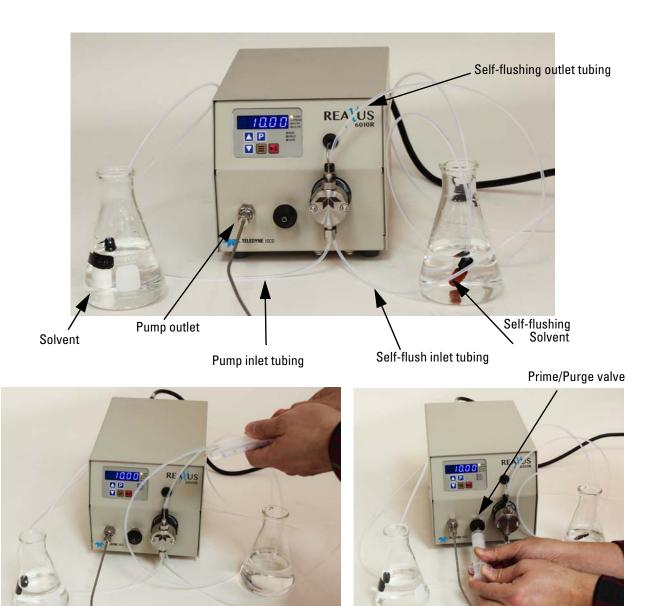
Figure 2-1 Starting the pump
