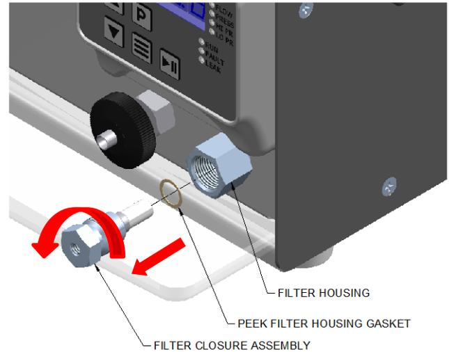
2. Install the new filter housing gasket onto the closure assembly and install into the filter housing making sure the gasket remains on the shoulder of the closure when installing into the filter housing, tightening by hand. Use a 5/8" wrench to hold the filter housing and torque the new filter closure assembly into the filter housing to 180 in\*lbs, or 1/4 turn past hand tight.
