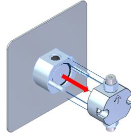
3. Carefully pull the flush housing forward and off the guide pins. Pull straight and slowly to prevent damage to the piston. **Note:** assure that the "O"-ring remains in the flush housing.
