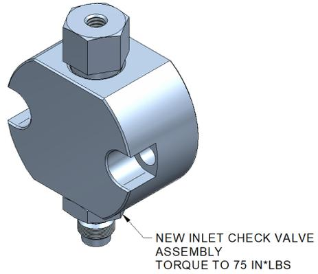
4. Customer supplied 1/8"OD tubing can now be connected to the inlet of the pump. \*Note – minimum tubing ID for inlet of pump should not be less than 0.085", or cavitation may occur.
