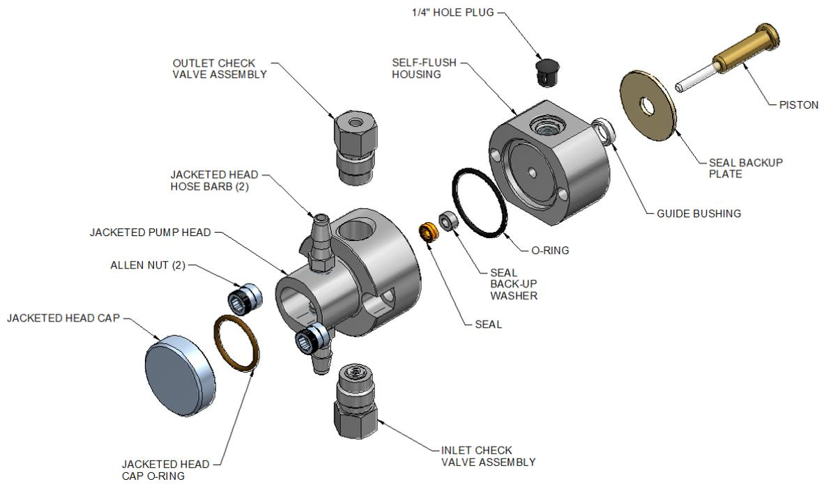
Figure 7. *Jacketed Hastelloy Non-Flushing Pump Head Assembly*
