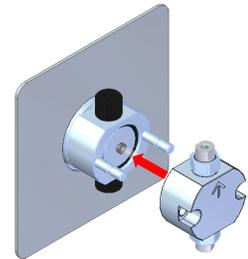
10. Using a hex tool, reinstall fasteners. As you tighten, alternate side-to-side until snug. Turn 1 flat past snug.
