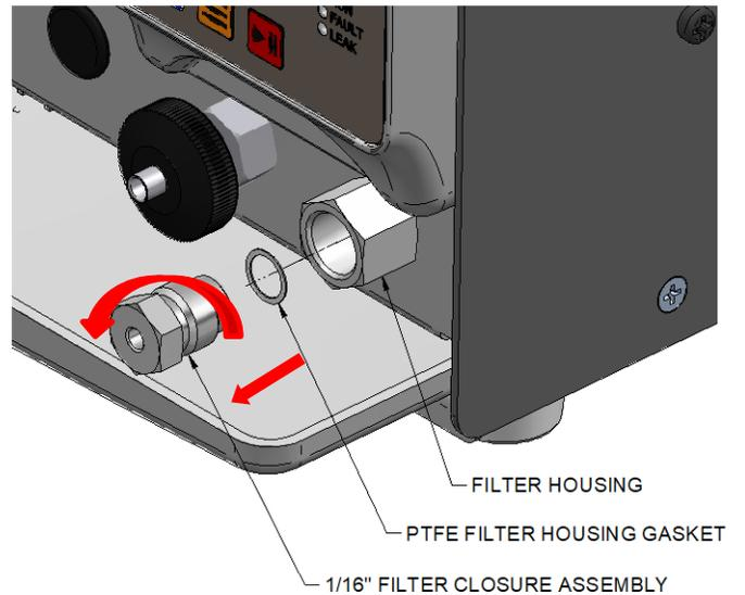
2. Install the new filter housing gasket onto the closure assembly and install into the filter housing making sure the gasket remains on the shoulder of the closure when installing into the filter housing, tightening by hand. Use a 5/8" wrench to hold the filter housing and torque the new filter closure assembly into the filter housing to 180 in\*lbs, or 1/4 turn past hand tight.
