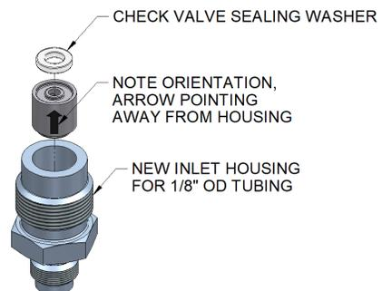
3. Install new check valve assembly into the inlet of the pump head. Torque the check valve housing to 75 in-lbs.
