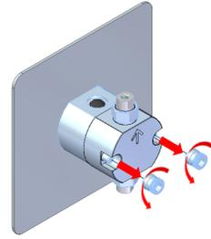
2. Carefully pull the pump head forward and off the guide pins. Keep the self-flush in place. Pull straight and slowly to prevent damage to the piston. **Note:** the back-up washer may remain on the piston. Carefully remove it and install when reassembling.
