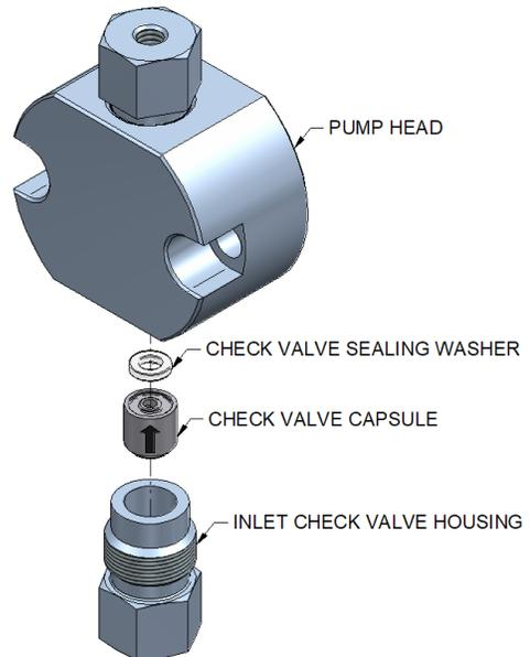
2. Install the check valve capsule into the new 1/8" OD tubing inlet housing as shown.
