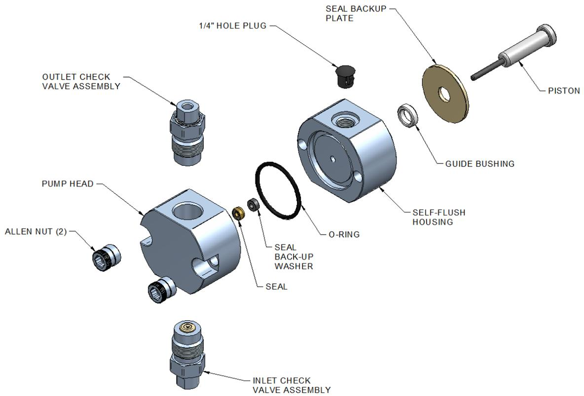
Figure 6. *Stainless Steel Non-Flushing Pump Head Assembly*
