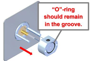
4. Using the supplied seal tool, remove the guide bushing in the direction shown. The outlet port hole plug can also be removed at this time.
