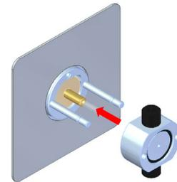
9. Carefully slide the back-up washer onto the piston, in front of the wash housing. Then, carefully slide the pump head into place. Push onto guide pins straight and slowly to prevent damage to the piston.
