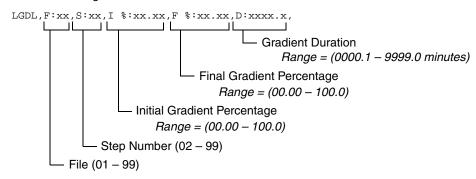
Figure 6-5 Gradient Download Commands - Single pump flow gradient
