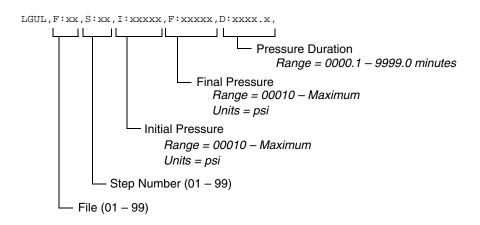
Figure 6-9 Upload Commands - Single pump pressure programming
