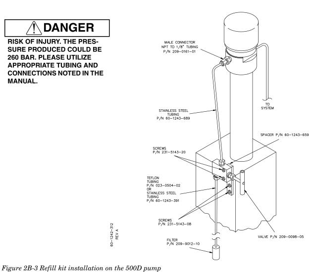
4. Then connect the PTFE tubing (with the filter) to the bottom port of the valve, using the valve fittings,
