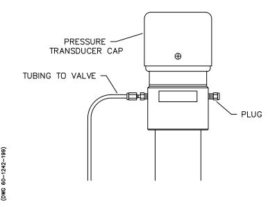
Figure 2B-1 Liquid system plumbing connections for the 500D pump
