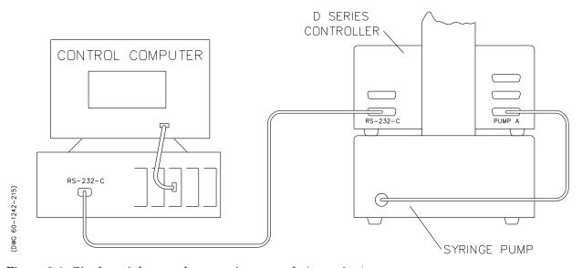
Figure 6-1 Single serial network connection example (rear view)
