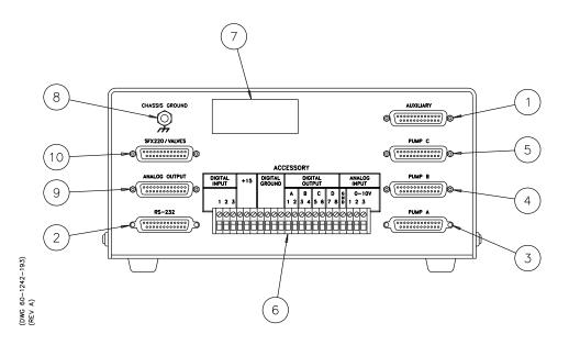
Figure 1-6 Pump controller rear panel connectors
