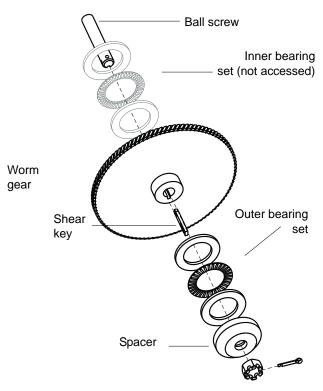
Figure 5-6 65DM Shear key replacement
