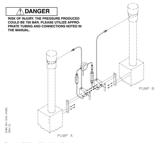
Figure 9-1 Modifier addition kit installation
