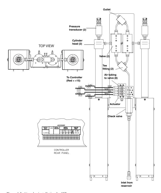
Figure 8-5 Air valve installation for 65D pump
