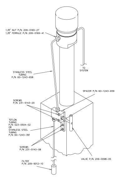
Figure 2A-4 Refill kit installation
