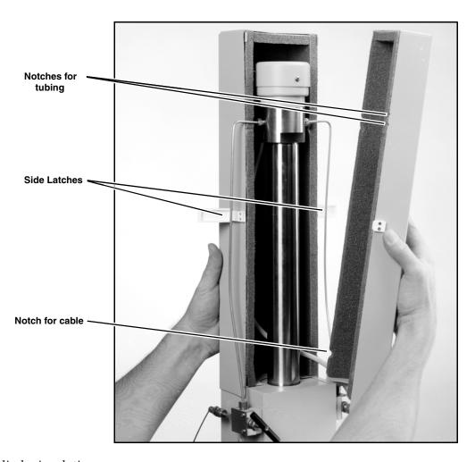
Figure 2D-3 Cylinder insulation cover
