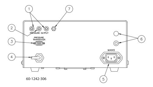
Figure 1-7 Pump rear panel connectors
