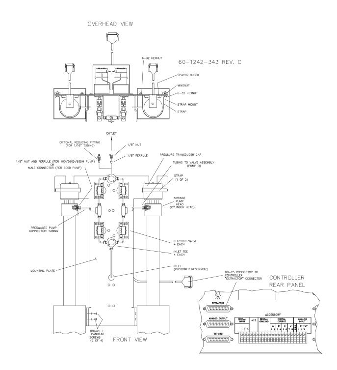
Figure 8-6 Electric valve installation
