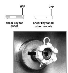
Figure 5-4 Shear key replacement
