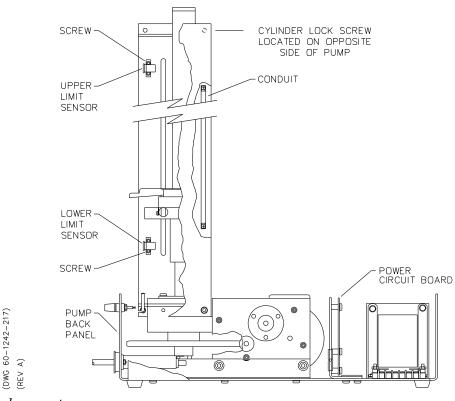
$Figure\ 5\text{-}10\ Limit\ sensor\ replacement$
