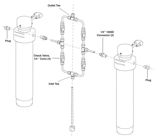
Figure 8-2 Check valve package installation: 1000D pump
