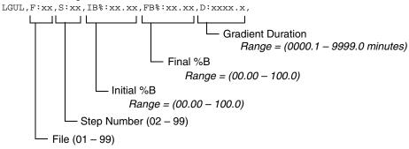
$Figure \ 6-8 \ \ Gradient \ Upload \ Commands - Two \ pump \ flow \\ gradient$
