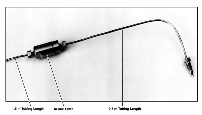
Figure 2A-7 In-line filter package
