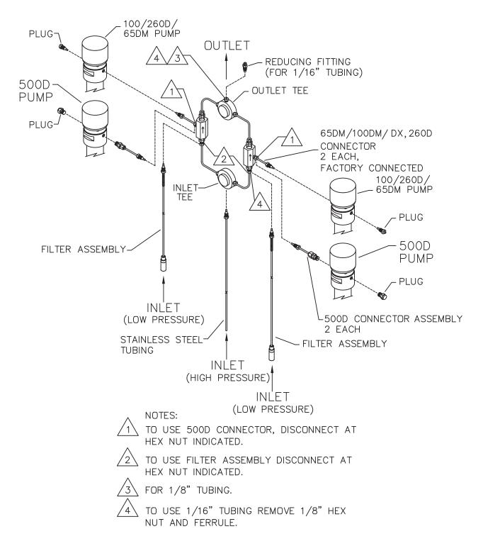
Figure 8-1 Check valve package installation: 65DM/100D/265D/500D pumps
