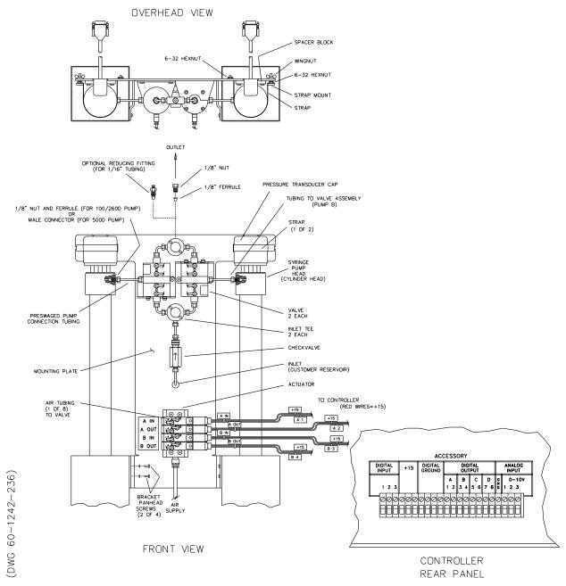
Figure 8-3 Air valve installation for 65DM, 100DM/DX, 260D, and 500D pumps
