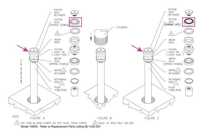
Figure 5-2 Break-in procedure for aqueous seals
