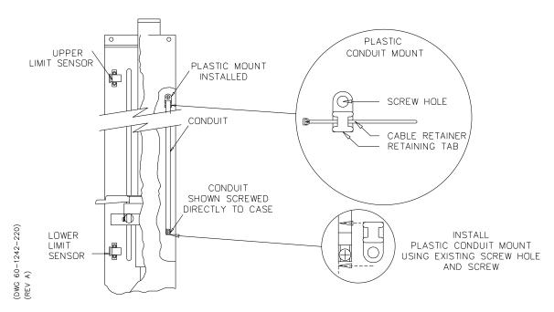
Figure 5-11 Installing the plastic mounts
