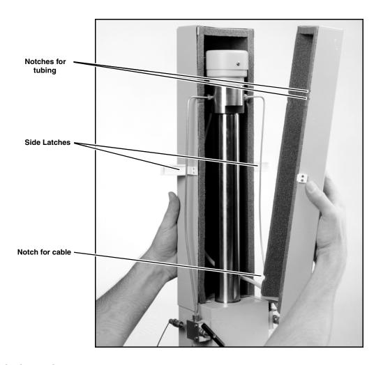
Figure 2A-8 Cylinder insulation cover
