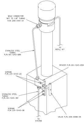
Figure 2B-4 500D pump outlet valve package installation
