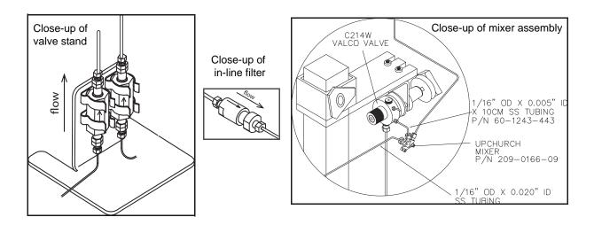
Figure 7-4 Dual gradient connections: Detail
