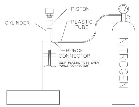
$Figure\ 2B\text{-}6\ Purge\ connector\ installation$
