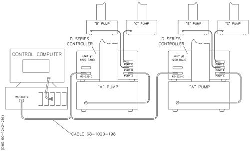
Figure 6-2 Serial network connection example
