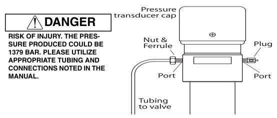
Figure 2D-1 Liquid system plumbing connections
