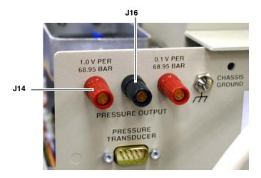
Figure 5-9 Pressure output jacks, pump rear panel
