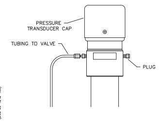
Figure 2C-1 Liquid system plumbing connections for the 1000D pump
