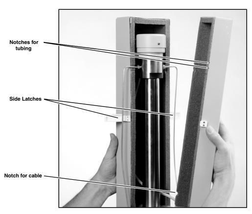
Figure 2B-5 500D cylinder insulation cover
