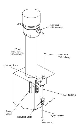
Figure 7-2 Pump outlet connections
