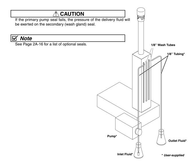
Figure 2C-3 1000D wash fluid connections
