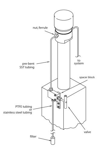
Figure 7-1 Pump inlet connections
