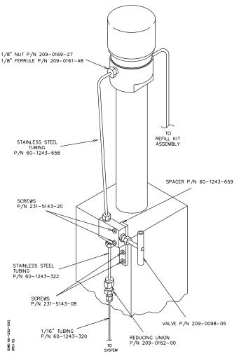
Figure 2A-6 Outlet valve package connection
