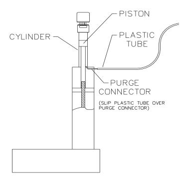
Figure 2A-11 Purge connector installation
