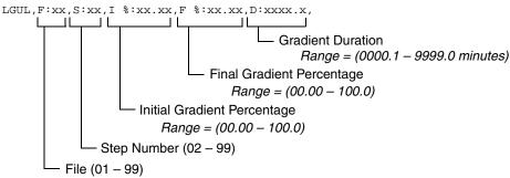
$\begin{tabular}{ll} Figure~6-7 & Gradient~Upload~Commands~-~Single~pump\\ flow~gradient \end{tabular}$
