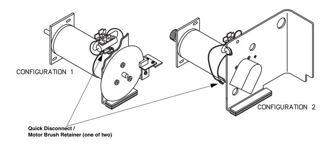
Figure 5-7 D Series motor brush replacement
