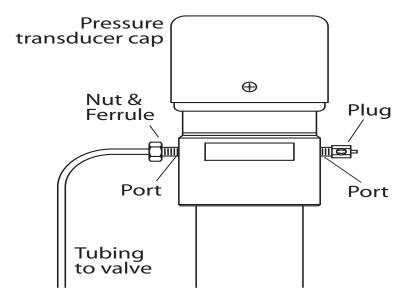
Figure 2A-1 Liquid system plumbing connections
