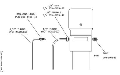
Figure 2A-2 Accessory package installation
