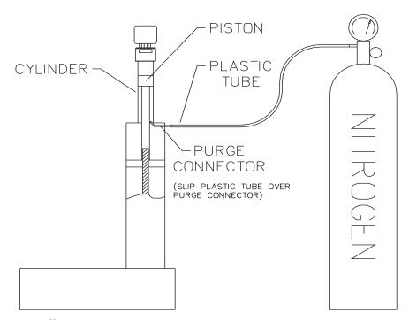
$Figure\ 2D\text{-}5\ Purge\ connector\ installation$
