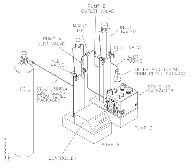
Figure 9-2 Two pump modifier system
