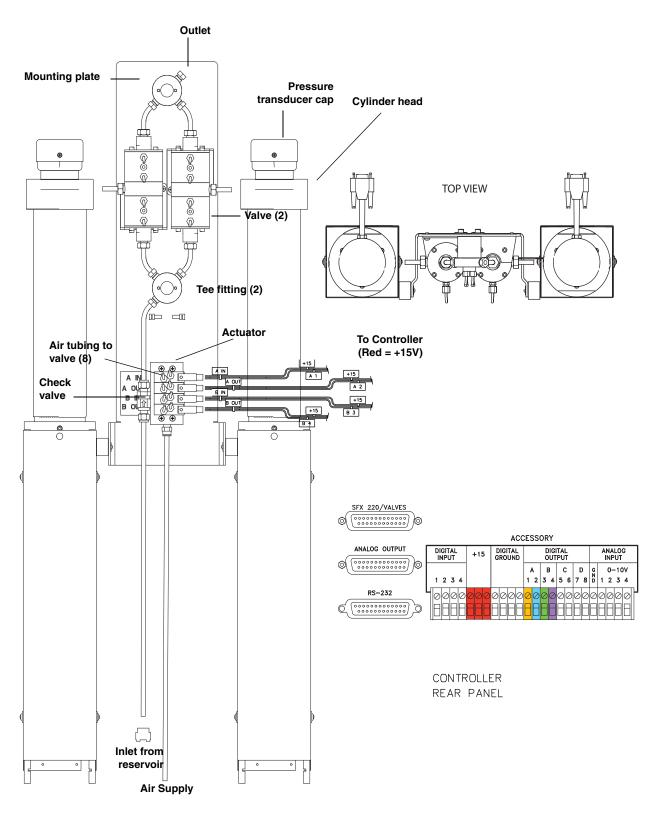
Figure 8-4 Air valve installation for 1000D pump
