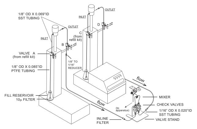
Figure 7-3 Dual gradient system connections (Inlet valves (A & C) are from refill valve kits)
