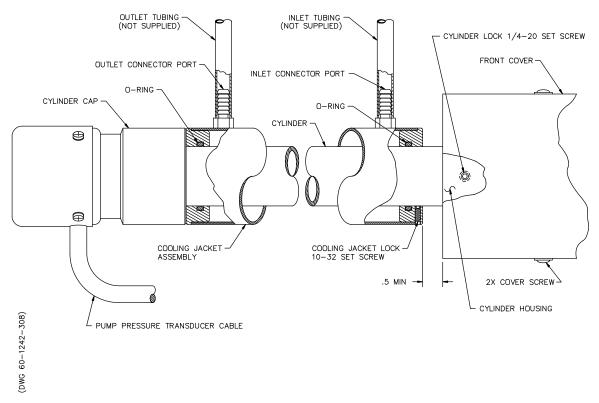
Figure 2D-4 Cooling/Heating jacket installed
