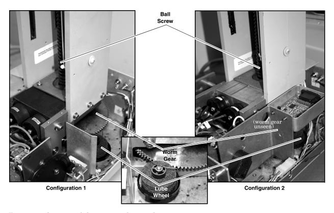
Figure 5-1 Gear train lubrication and motor drive service
