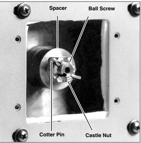
Figure 5-3 Accessing the shear key
