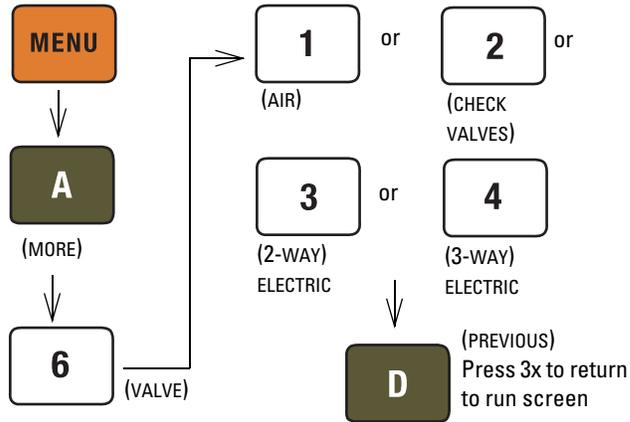
Figure 5-4 Keystrokes to specify valve type
