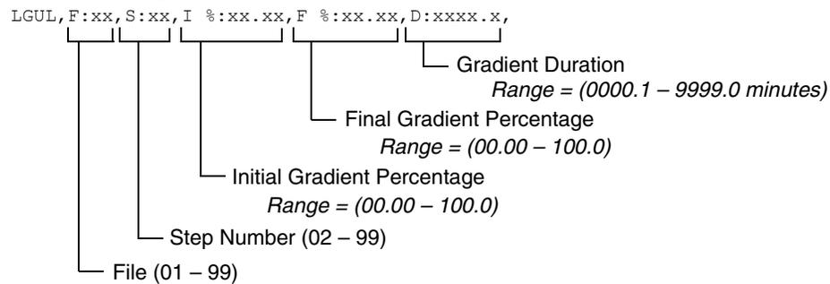
Figure 7-9 Gradient Upload Commands - Single pump flow gradient
