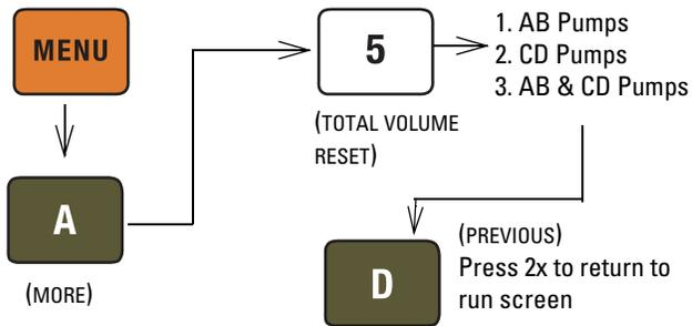
Figure 5-5 Keystrokes to reset volume totalizer
