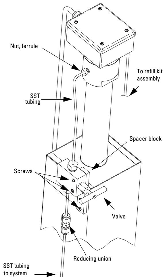
Figure 4-2 Pump outlet connections
