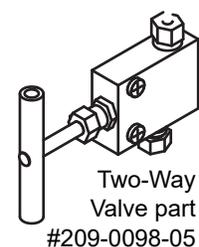
Following installation, the tubing connections must be tested for leaks before any program is run. If a leak is found, tighten the connection slightly. If the leak persists, swage the connection again with a new ferrule. Refer to Technical Bulletin [TB05 Field Verification Procedures](http://www.isco.com/sp_applications/#techbulletins) at [http://www.isco.com/sp\\_applications/#techbulletins](http://www.isco.com/sp_applications/#techbulletins) for leak test procedures.
