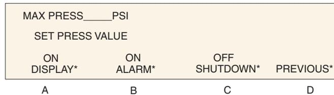
Figure 3-9 Limits setpoint (Max Press) menu
