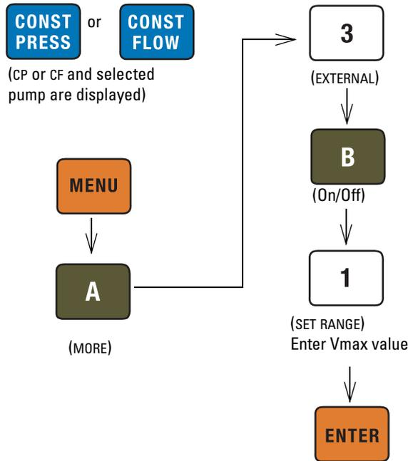
Figure 3-13 Button sequence for external control setup
