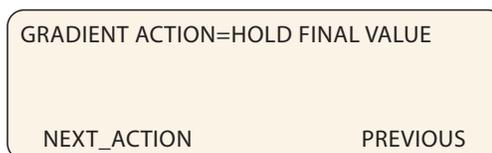
To scroll through the four options, press NEXT\_ACTION (A). When you have reached the desired option, press PREVIOUS (D) to save and exit.
