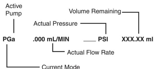
**Line Two** – The second line varies slightly depending on the operating mode. A file or step will only be displayed when operating in the gradient mode.
