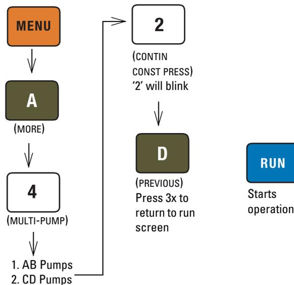
Figure 5-7 Keystrokes to set up constant pressure
