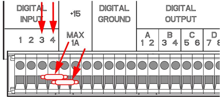
Figure 3-11 External resistor locations
