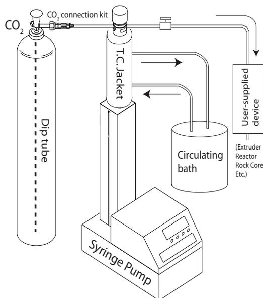
Figure 2-8 System with temperature control jacket installed
