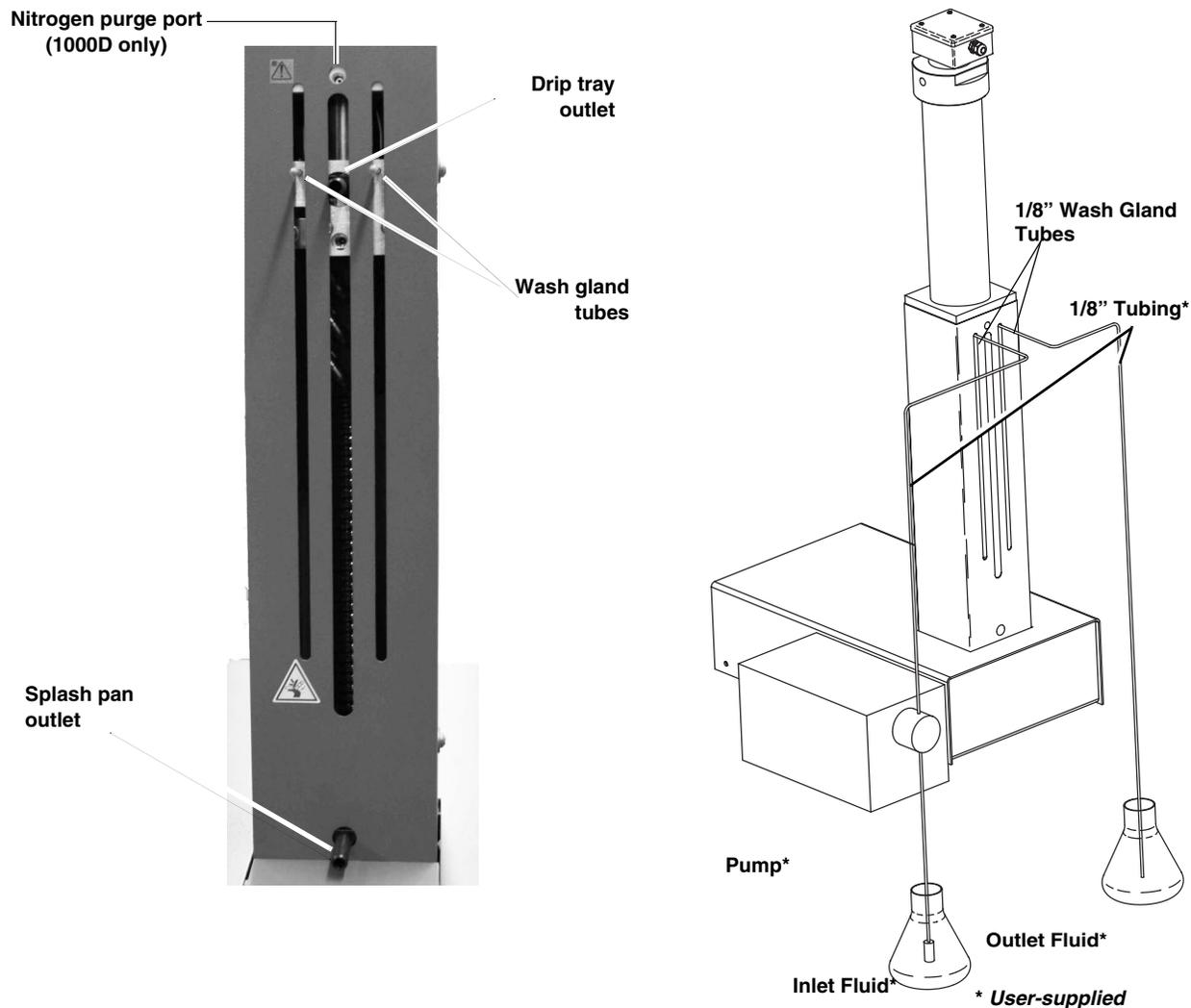
Figure 2-2 Drain tube installation and wash gland connection
