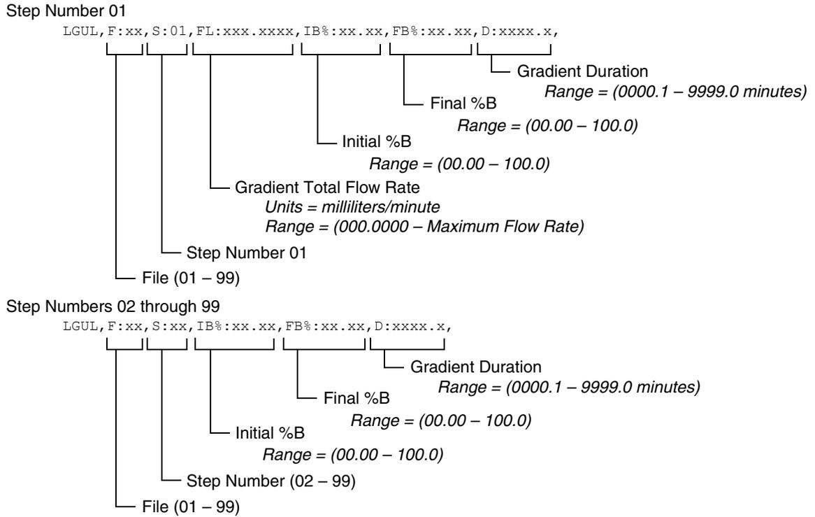
*Figure 7-8 Gradient Download Commands - Two pump flow gradient*
