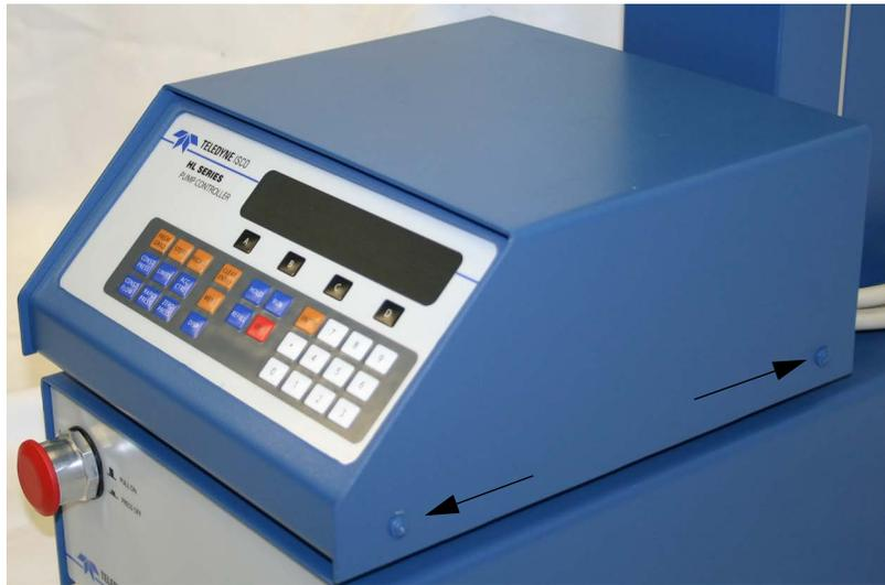
Figure 8-5 Controller case top screws (2 of 4 shown)
