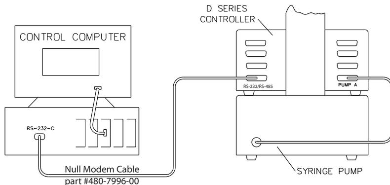
Figure 7-1 Serial network connection example - Single connection
