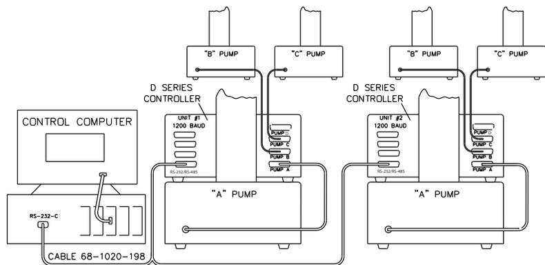
Figure 7-2 Serial network connection example - Dual connection
