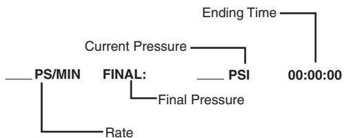
**Line Four** – Line four varies depending on the mode. The options presented on this line are softkey selectable, *i.e.* you use the softkeys (A - D) located under the screen to choose the option.
