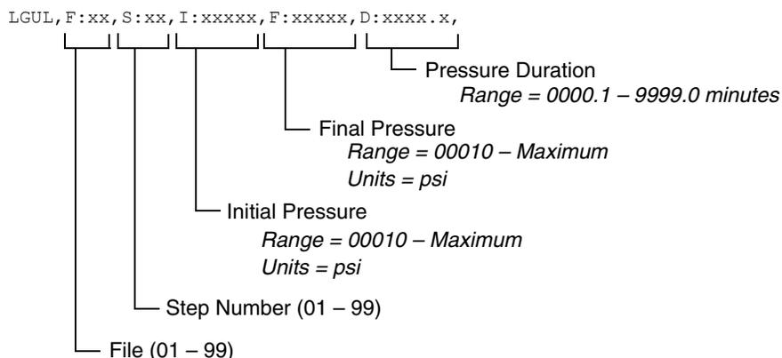
Figure 7-11 Upload Commands - Single pump pressure programming
