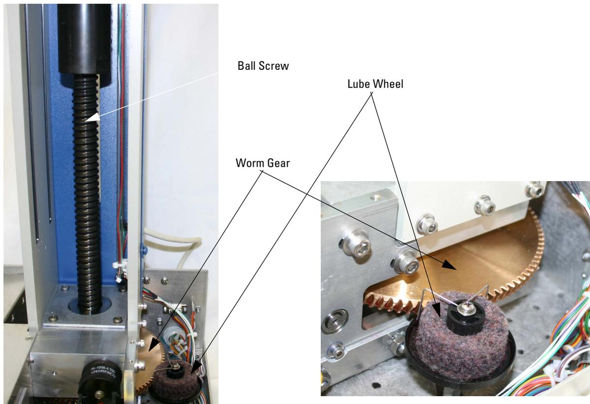
Figure 8-7 Gear train lubrication and motor drive service
