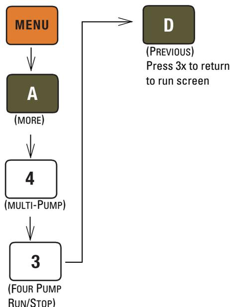
Figure 5-8 Keystrokes to Run or Stop the pumps
