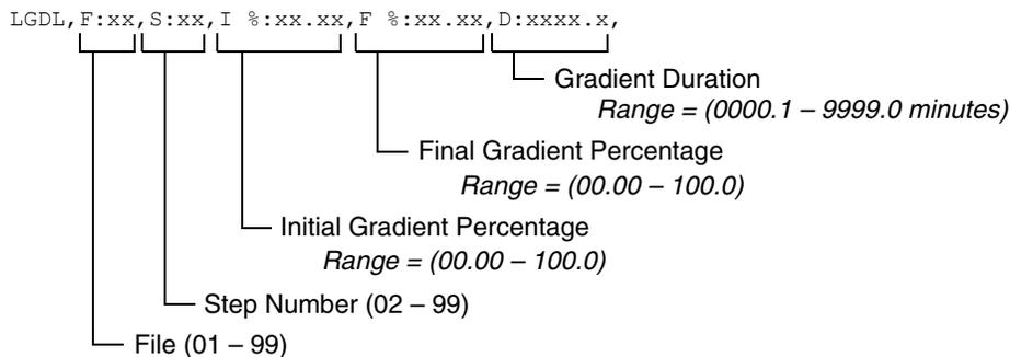
Figure 7-7 Gradient Download Commands - Single pump flow gradient
