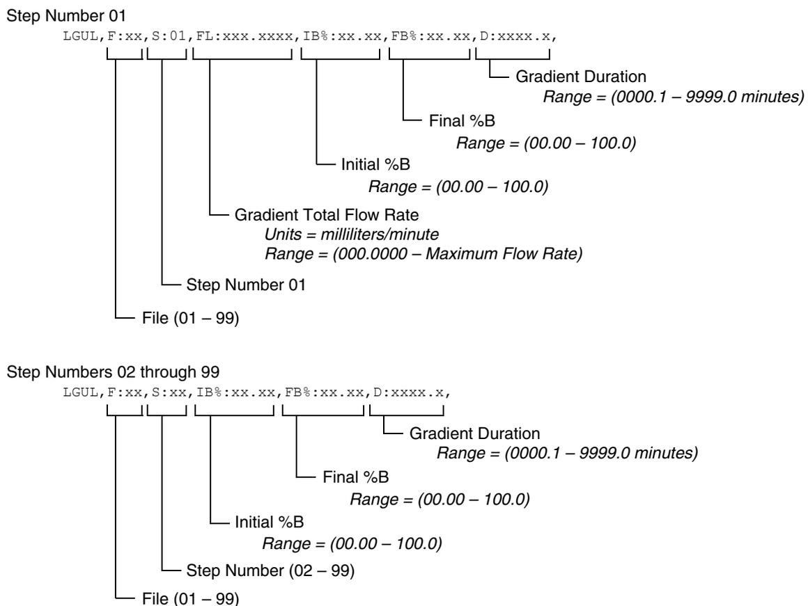
*Figure 7-10 Gradient Upload Commands - Two pump flow gradient*
