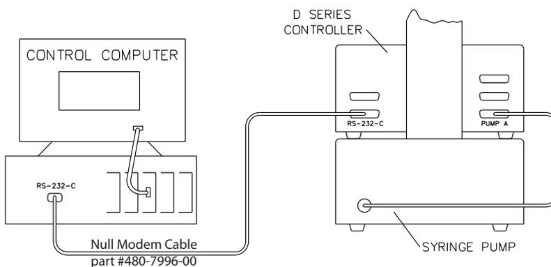
Figure 8-4 Serial connection to a computer
