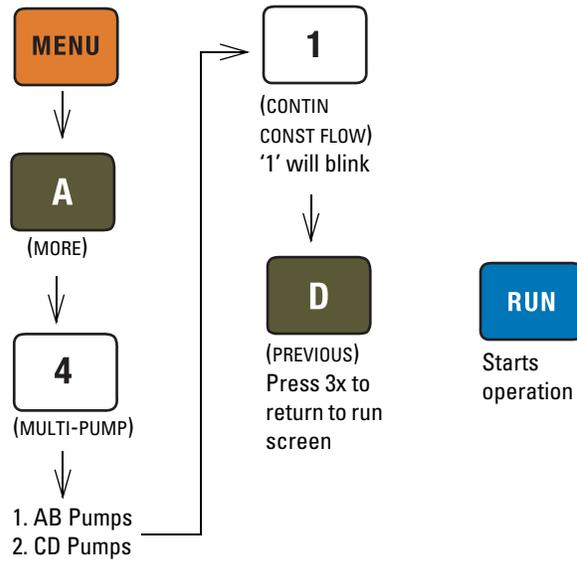
Figure 5-6 Keystrokes to set up constant flow
