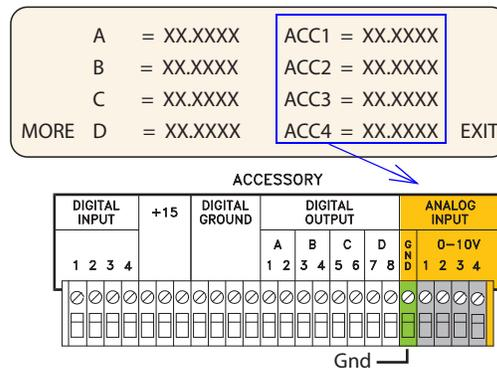
Figure 8-2 Analog Input diagnostic screen
