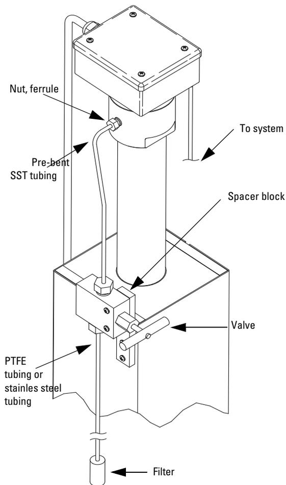
Figure 4-1 Pump inlet connections
