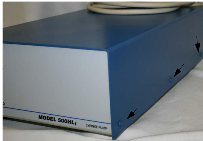
Figure 8-6 Pump case top screws (3 of 6 shown)
