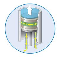
The 1000x includes a seal and cylinder wash feature that allows a rinse solution to be circulated between the seals. This protects the seals and cylinder walls against abrasion from salt or other material that may crystallize or precipitate from the solution in the pump.
