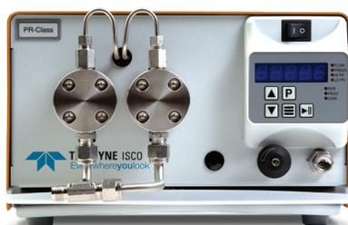
The pumps are designed for a wide range of Preparative and Semi-Prep Chromatography, as well as SMBC (simulated moving bed chromatography), and many process and industrial applications. With 100 mL/min and 300 mL/min versions, reaching pressures up to 4,000 psi, the pumps will meet the most demanding LC and process needs.
