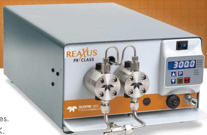
The rugged PR Class consists of dual-headed, positive displacement piston pumps that provide high, accurate flows and excellent pressure capability for a variety of uses. Standard fluid path materials are Stainless Steel and PEEK.
