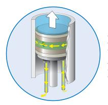
The 1000D includes a seal and cylinder wash feature that allows a rinse solution to be circulated between the seals. This protects the seals and cylinder walls against abrasion from salt or other material that may crystallize or precipitate from the solution in the pump.
