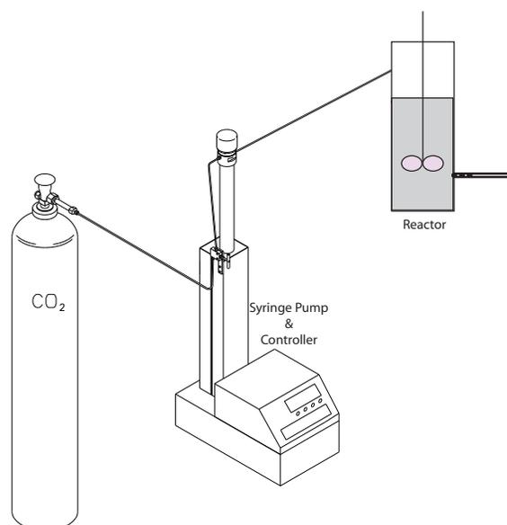
**Figure 2: Configuration for pressure control of SFCO<sub>2</sub> density and solubility during reaction**
