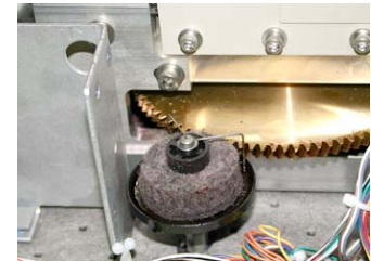
Figure 5: Lube wheel (Saturate with ALMASOL 609)
