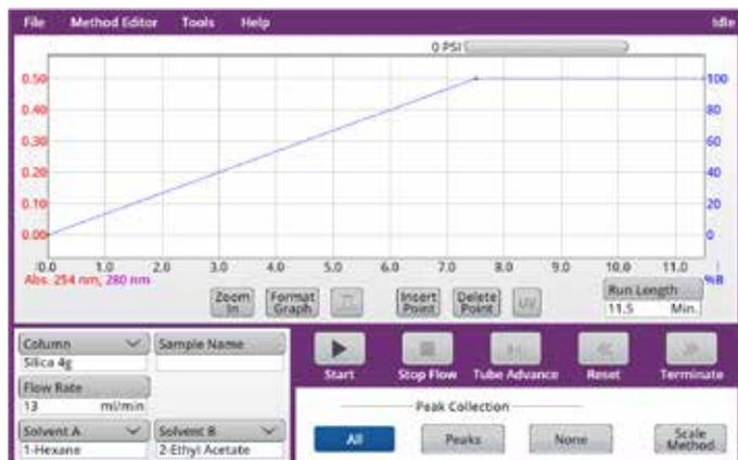
Figure 4: Main Separation Window
