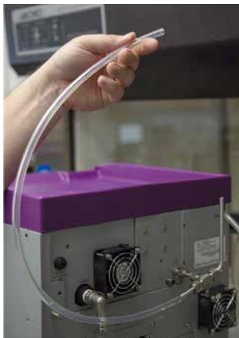
Figure 3: Filling the P-trap drain. Keep liquid level lower than the top of the system
