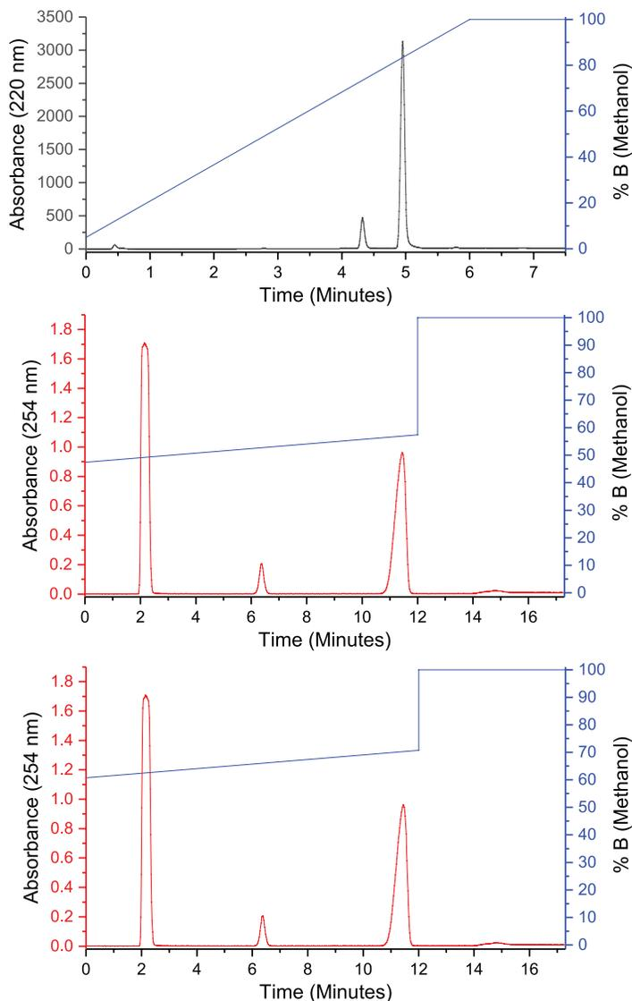
**Figure 2—Analytical scouting runs and focused gradients on a C18 column, using the C8 column calibration. The first preparative run was focused on the compound eluting at 4.324 minutes in the analytical run, while the peak at 4.953 minutes was used to calculate the second preparative gradient.**
