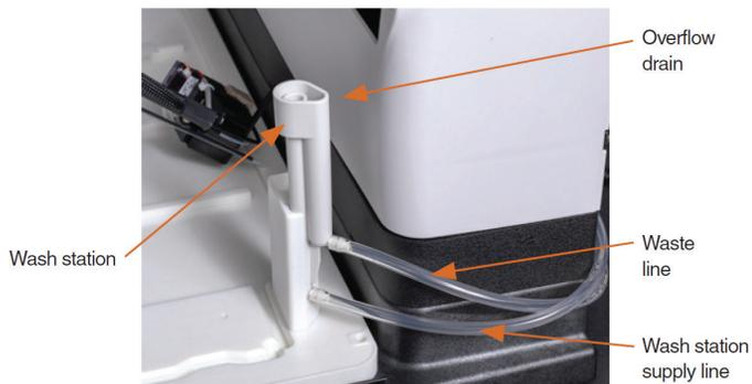
**Figure 3: Wash station and overflow drain**
