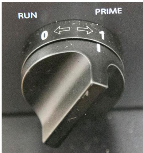
Figure 1: Turn the valve to the Prime position
