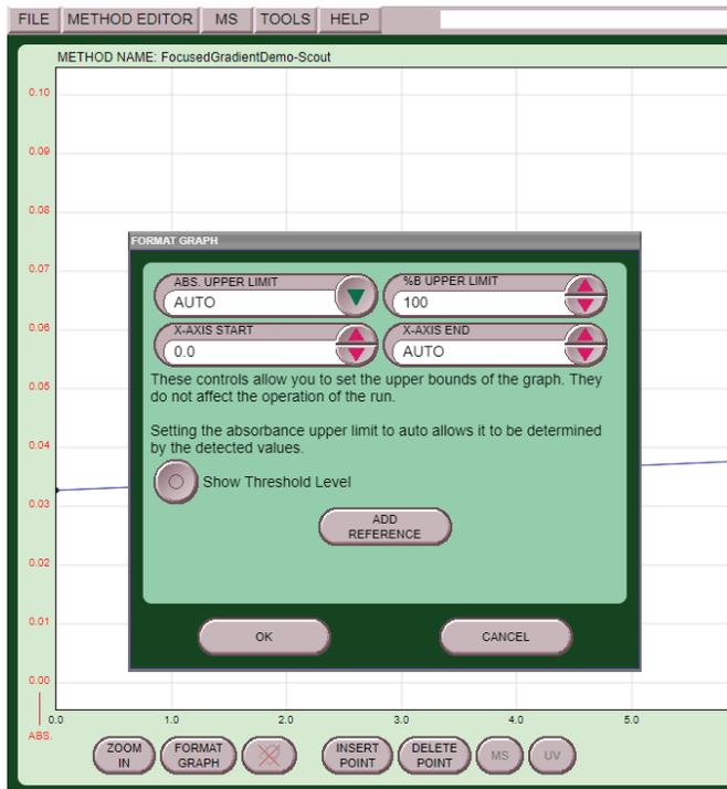
Figure 9: Format Graph screen to add a reference chromatogram
