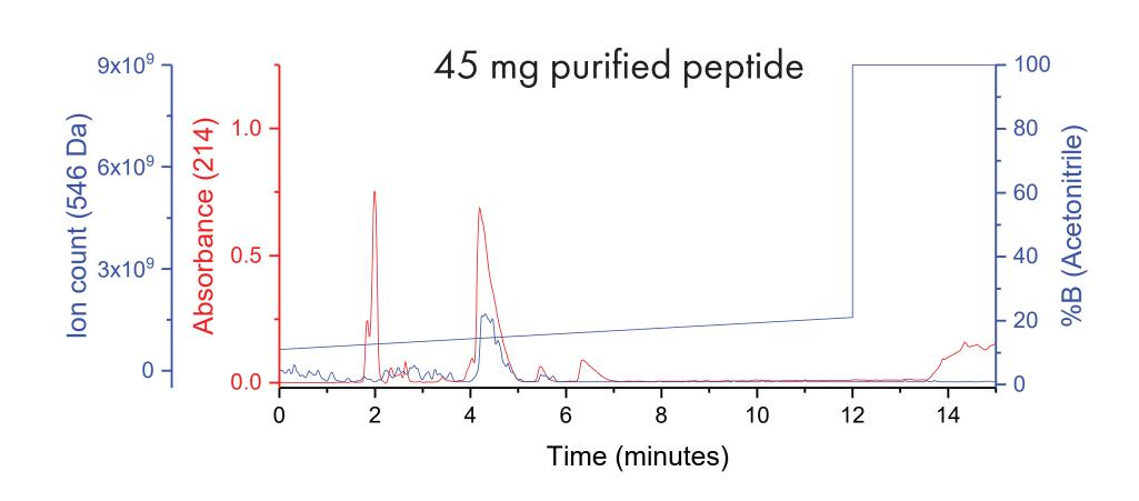
Injection of peptide dissolved in water. Peptide was pre-purified on a flash system prior to final purification on the ACCQPrep system.
