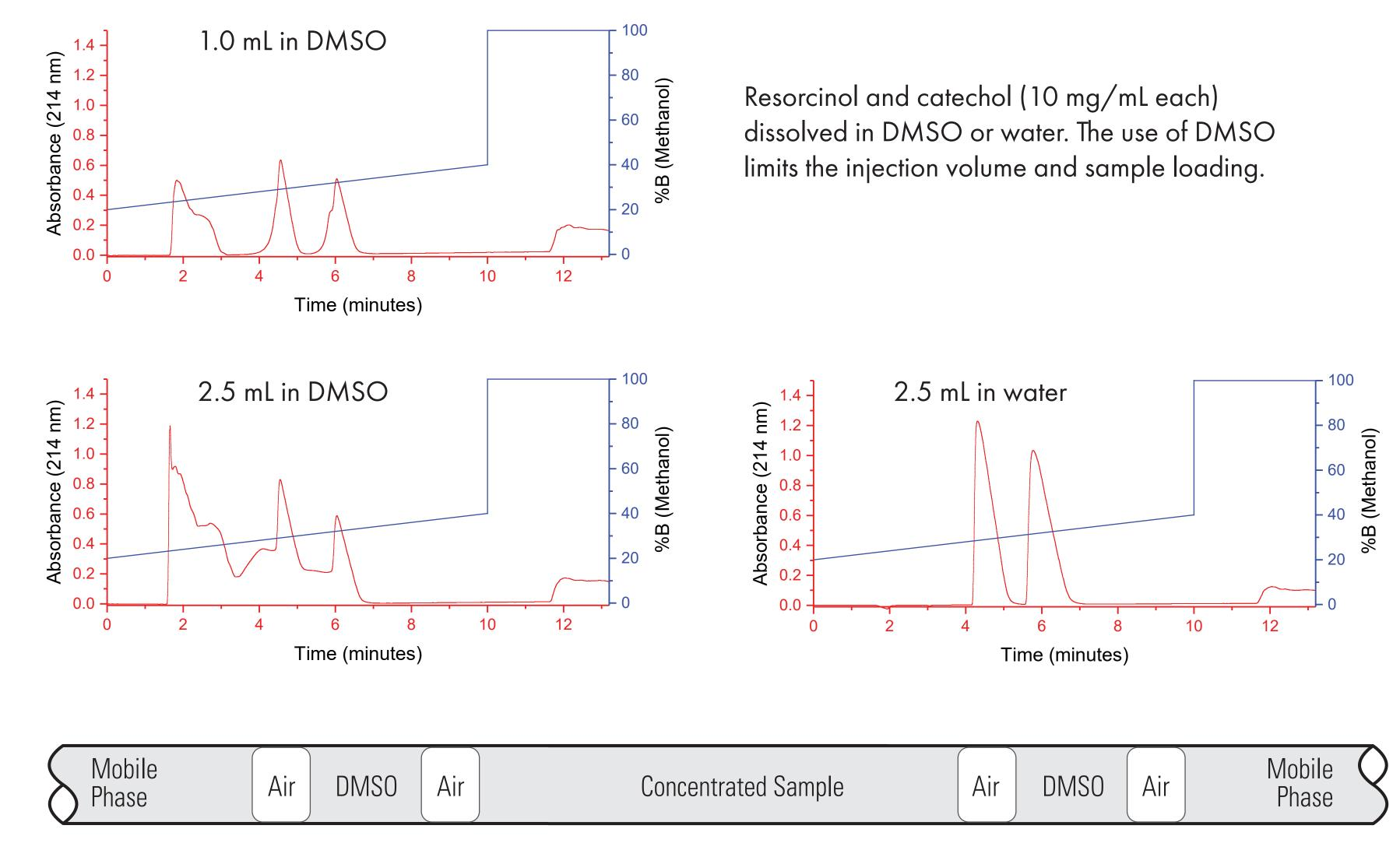
Tube cross section showing DMSO slugs with air gaps. On-column dilution replaces the DMSO with water. Precipitation is prevented because of the air gaps.
