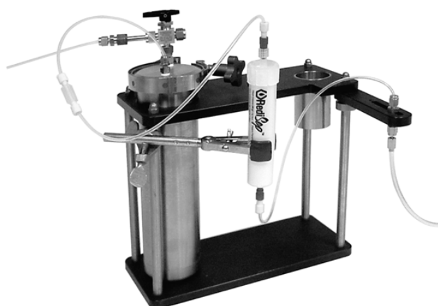
Figure 1: RediSep column on pressurized solvent reservoir system
