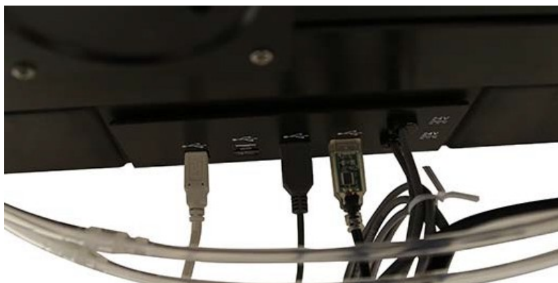
Figure 3-16 AutoSampler Module USB-A connection (center)
