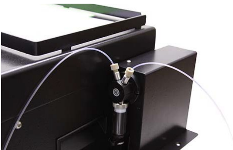
Figure 4-22 Waste line connected to the right AutoInjector Module port
