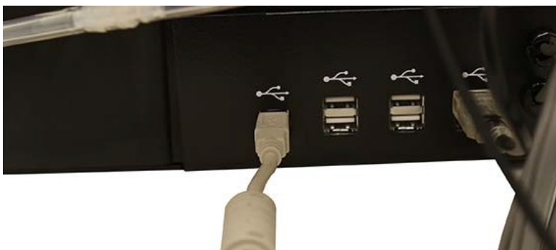
Figure 3-24 AutoSampler Module USB-B connection
