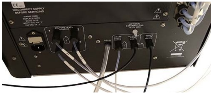
Figure 3-26 Diverter Valve Waste port with AutoSampler Module tubing connection
