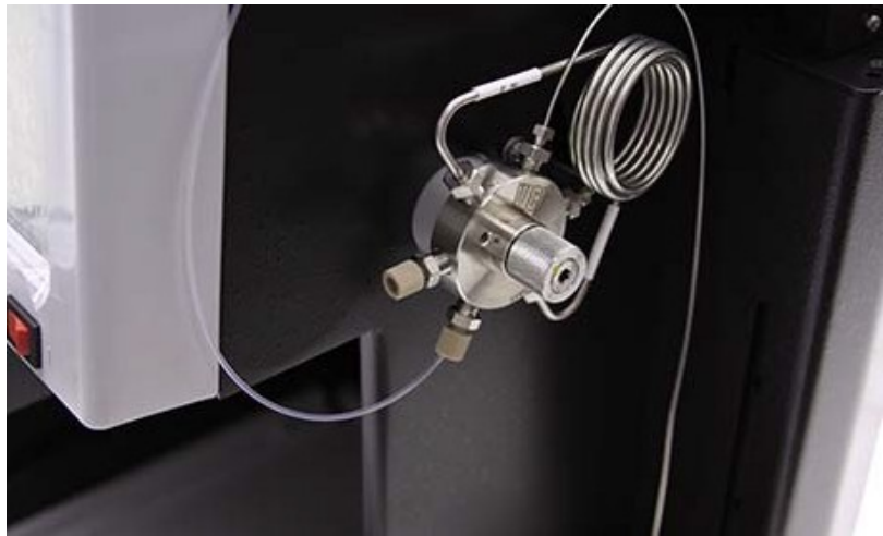
Figure 2-11 Sample tube fitting attached to the EZ Prep inject valve
