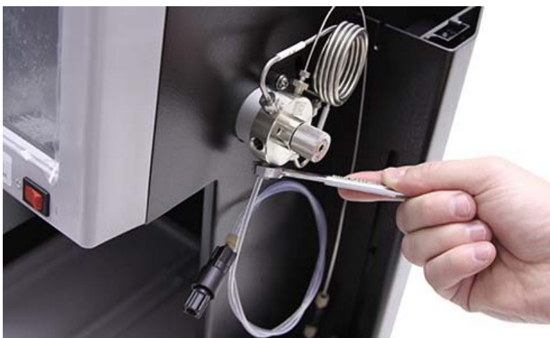
Figure 2-3 Removing the waste line from the EZ Prep inject valve
