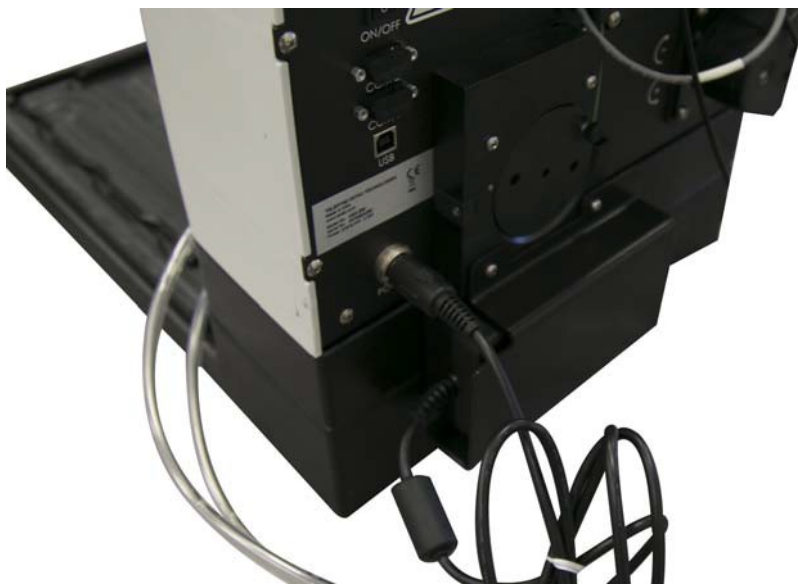
Figure 3-22 AutoSampler Module with power connection made
