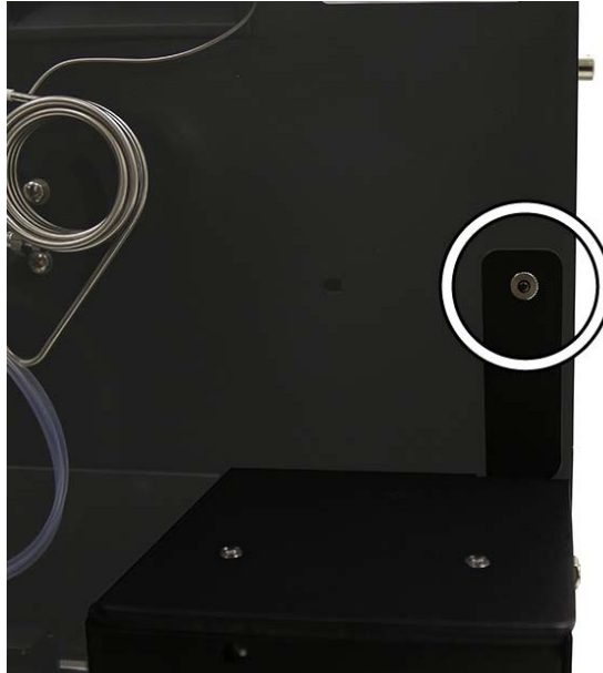
Figure 4-8 Location of the Column Selector Module mounting rail attachment thumbscrew
