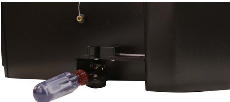
Figure 4-2 Removing the bottom section housing nut
