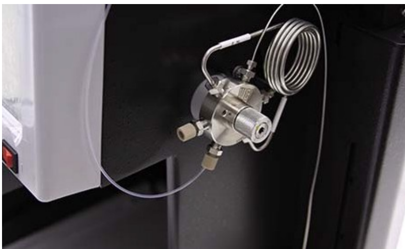
Figure 4-24 Sample tube fitting attached to the EZ Prep inject valve
