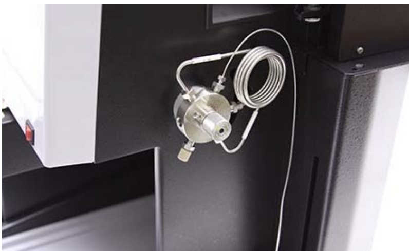
Figure 4-18 Waste tubing fitting attached to the EZ Prep inject valve
