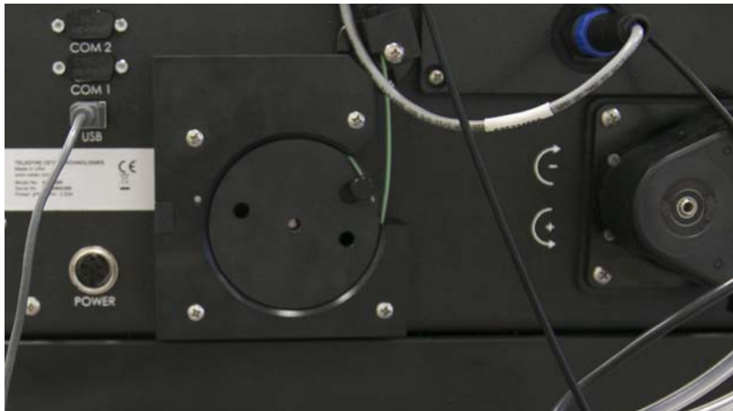
Figure 3-18 AutoSampler Module rotor before removing the bottom screws
