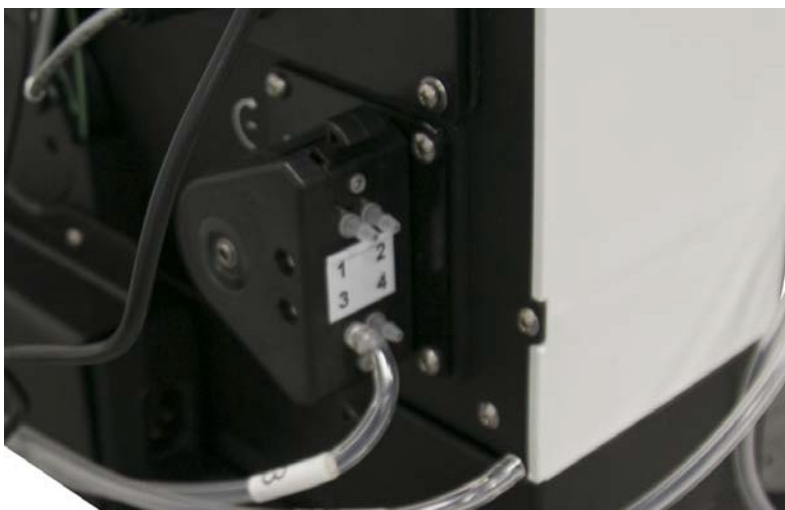
Figure 3-9 Routing the bottom section of wash station tubing
