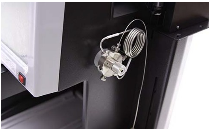
Figure 4-19 Waste fitting with the plastic fitting removed
