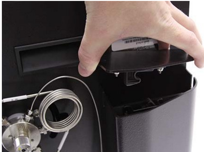
Figure 2-1 Removing the top cover of the EZ Prep column mount
