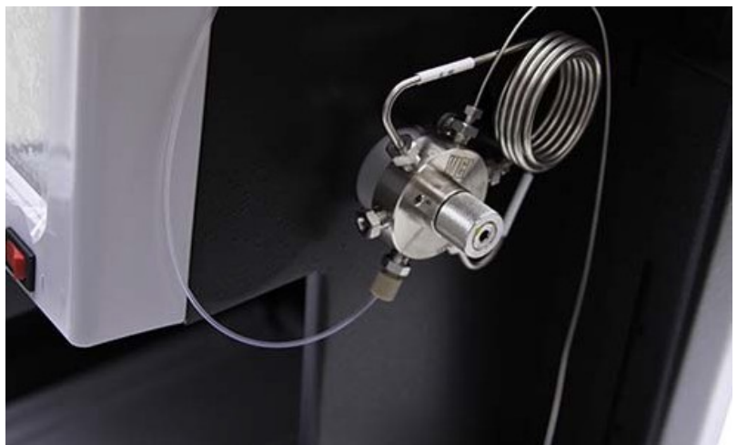
Figure 2-12 Sample probe tube fitting with the plastic fitting removed
