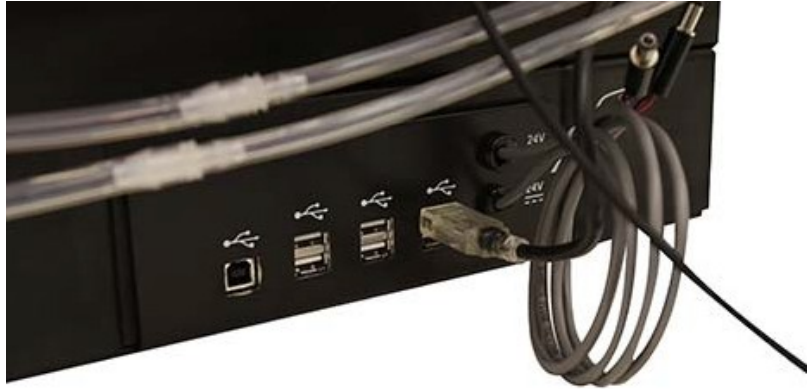
Figure 3-14 AutoSampler Module USB-A connection
