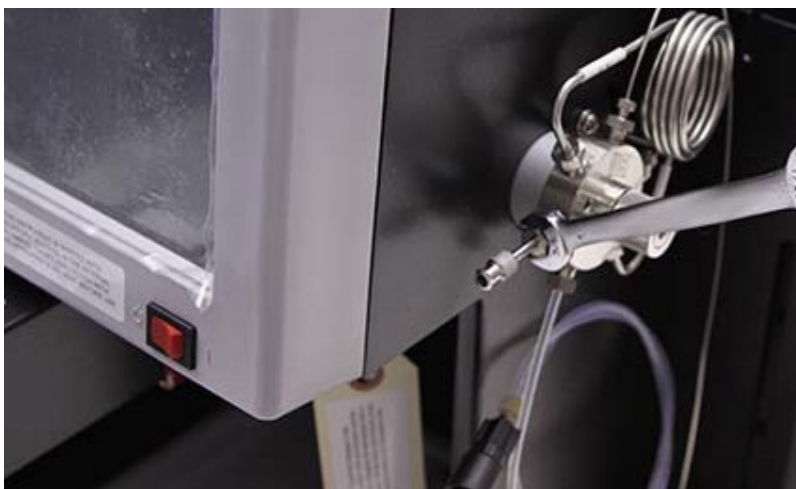
Figure 2-2 Removing the Luer fitting from the EZ Prep inject valve
