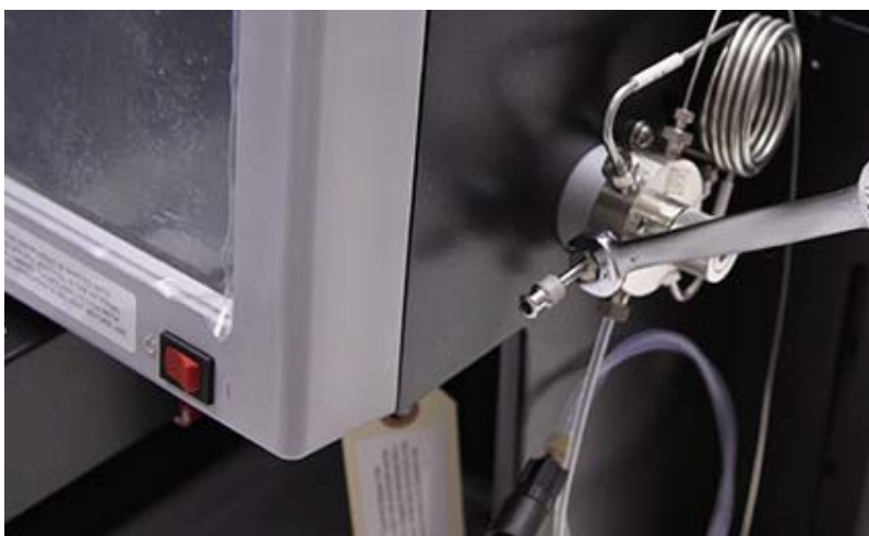
Figure 4-16 Removing the Luer fitting from the EZ Prep inject valve
