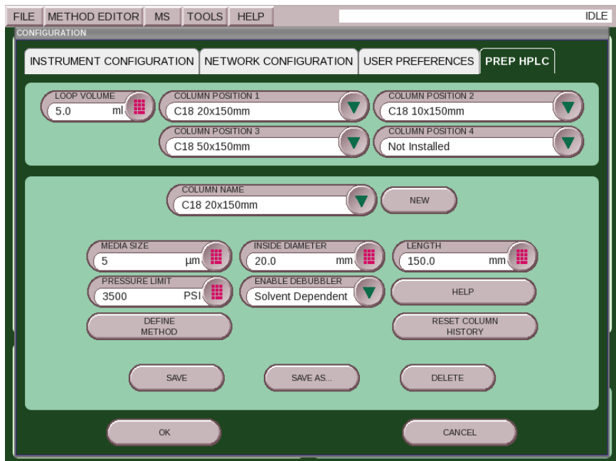
Figure 4-27 Configuring the Prep HPLC tab
