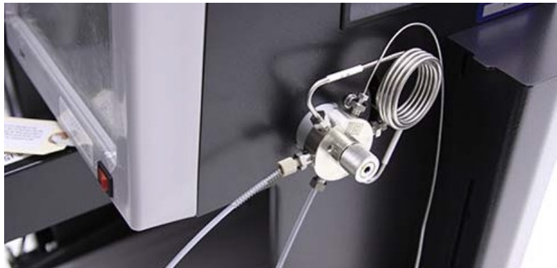
Figure 3-30 Sample probe tube fitting with sample probe tubing attached
