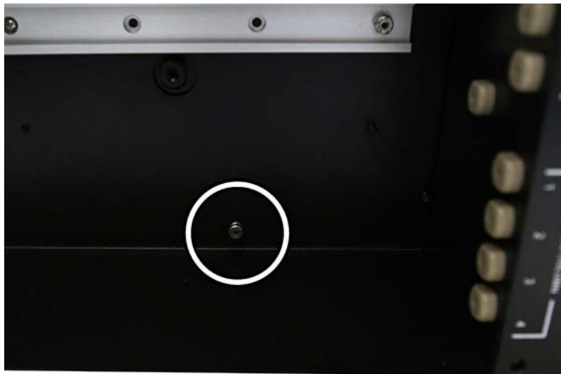
Figure 4-9 Location of the Column Selector Module lower attachment thumbscrew
