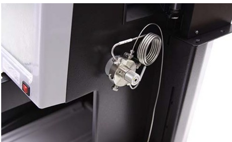
Figure 3-33 Waste fitting with the plastic fitting removed
