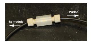
Figure 4-3 Coupler for connecting 4x tubing
