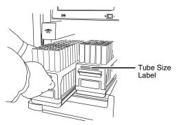
Figure 2-8 Inserting the collection tube rack
