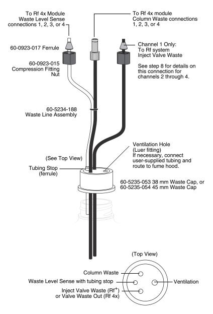
Figure 4-7 Recommended Rf 4x module channel 1 waste connections
