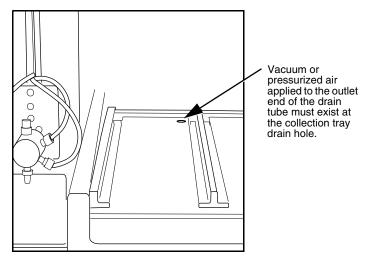
Figure 2-5 Fraction Collector Drain
