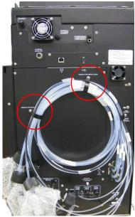
Figure 2-4 Remove the two shipping clamps indicated above
