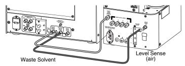
Figure 4-6 CombiFlash Rf system to Rf 4x waste tubing connections (all other connections not shown)
