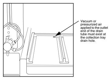
Figure 8-1 Collector tray drain hole
