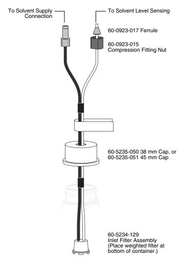
Figure 2-2 Recommended solvent connection
