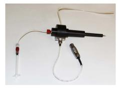
Figure 8-10 ESI probe with syringe
