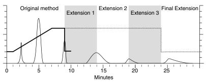
Figure 3-9 Automatic Run Extension Examples
