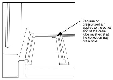
Figure 3-4 Fraction Collector Drain
