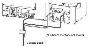
Figure 4-8 Channel 1 waste tubing connections
