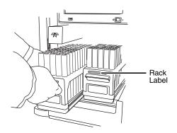
Figure 3-7 Inserting the collection tube rack
