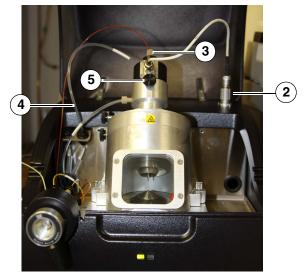
6. Pull out the ESI Probe directly up and out of the ion source chamber.
