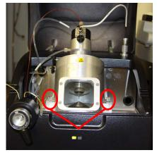
3. Gently lift and pull out the ion source chamber.
