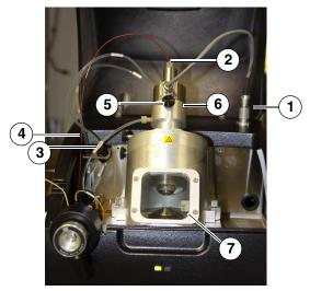
Figure 8-8 Removing the APCI probe
