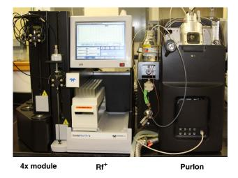
Figure 4-2 Component arrangement for connection with Rf system, 4x module and PurIon
