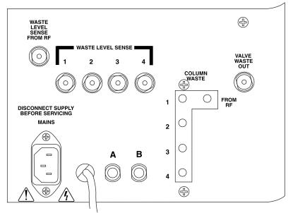
Figure 4-4 Rf 4x Module back panel connections
