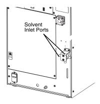
Figure 3-2 CombiFlash Rf150 solvent inlet ports
