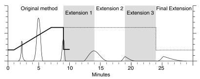
Figure 2-10 Automatic Run Extension Examples
