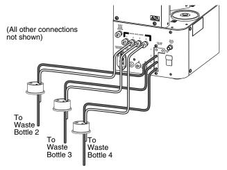
Figure 4-9 Channels 2 through 4 waste tubing connections
