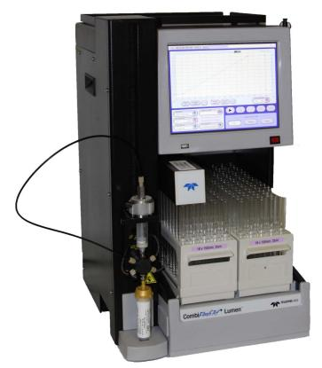
Figure 1-3 CombiFlash Rf<sup>+</sup> Lumen system, with evaporative light scattering and UV (or UV-vis) detection
