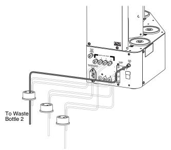
Figure 4-10 Valve Waste Out routed to Channel 2
