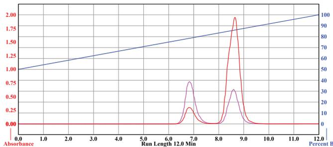
**Figure 2: Universal Verification Chromatogram for 275 g C18 column with MeOH/Water.**
