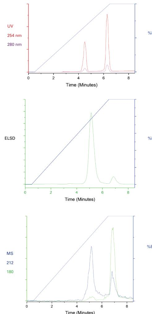
**Figure 1: Normal Phase Detector Response**
