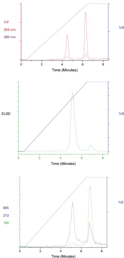
**Figure 1: Normal Phase Detector Response**
