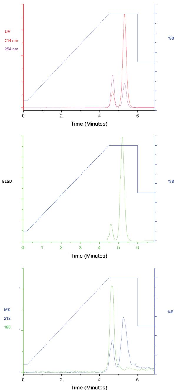
**Figure 2: Reverse Phase Detector Response**
