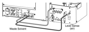
Figure 4-4 CombiFlash Rf system to Rf 4x waste tubing connections (all other connections not shown)
