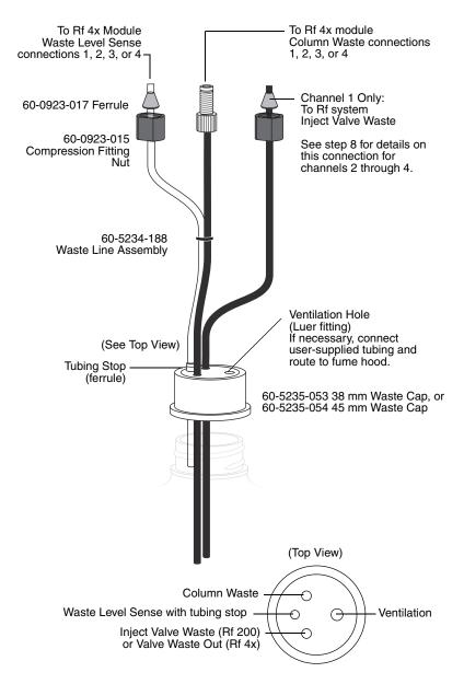
Figure 4-5 Recommended Rf 4x module channel 1 waste connections
