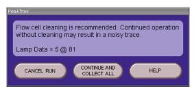
Figure 8-4 Flow cell cleaning message
