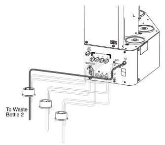
Figure 4-8 Valve Waste Out routed to Channel 2
