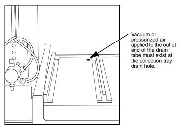
Figure 2-4 Fraction Collector Drain
