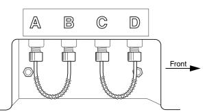
Figure 4-1 Labeled ports on CombiFlash Rf system side panel
