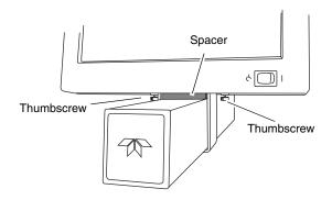
Figure 3-1 Remove arm stowing bracket and spacer
