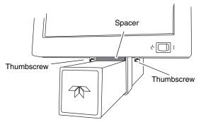
Figure 2-1 Remove arm stowing bracket and spacer
