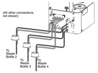
Figure 4-7 Channels 2 through 4 waste tubing connections
