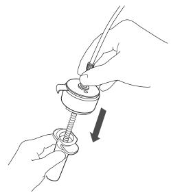
Figure 5-2 Insert the plunger to the bed
