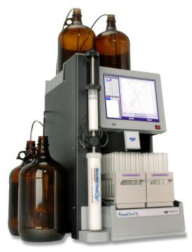
Figure 1-2 CombiFlash Rf 200 system, 5–200 mL/min, 200 psi (with automatic injection valve)
