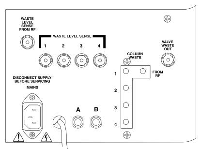
Figure 4-2 Rf 4x Module back panel connections
