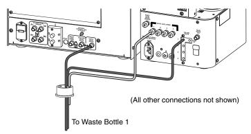
Figure 4-6 Channel 1 waste tubing connections
