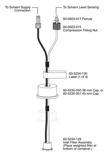
Figure 2-2 Recommended solvent connection
