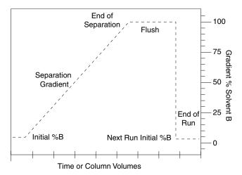
Figure 8-3 Default post-separation column and flow cell flush
