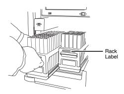
Figure 3-7 Inserting the collection tube rack
