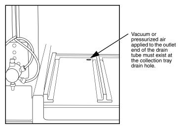
Figure 8-1 Collector tray drain hole
