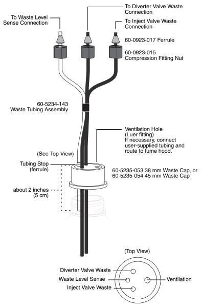
Figure 2-3 Recommended waste connections, with plastic plate
