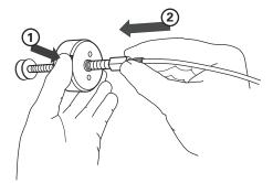
Figure 5-1 Press the lever and extend the plunger
