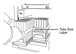
Figure 2-7 Inserting the collection tube rack
