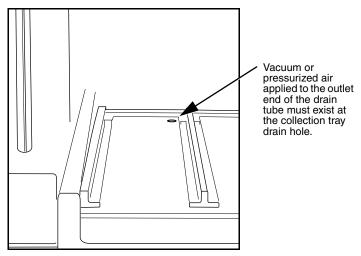
Figure 3-4 Fraction Collector Drain
