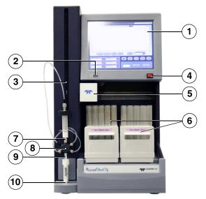
Figure 1-5 CombiFlash Rf Features (Front)
