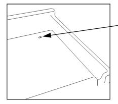
Vacuum or pressurized air applied to the outlet end of the drain tube must exist at the top self drain hole.
