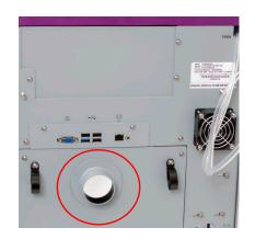
Figure 2-9 Location of the external exhaust port
