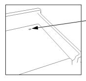
Vacuum or pressurized air applied to the outlet end of the drain tube must exist at the top shelf drain hole.
