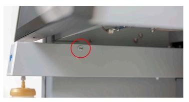
Figure 2-1 Remove screw holding the arm in place
