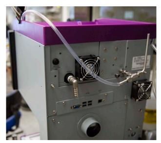
Figure 5-10P-trap pump drain line draped over the unit
