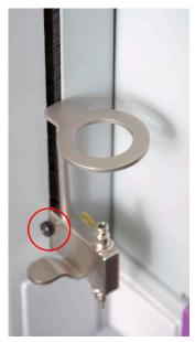
Figure 2-12 Location of the side hole to secure the SLCC ring support
