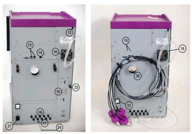
Figure 1-7 CombiFlash NextGen features (back)
