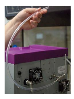
Figure 5-8 Line filled with 40 ml of acetone
