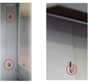
Figure 2-8 Location of holes for the vapor enclosure
