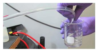
Figure 5-9 Draining the acetone into a 100 mL beaker
