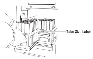
Figure 2-14 Inserting the collection tube rack
