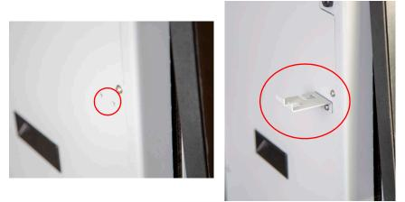
Figure 2-10 Before (left) and after SLCC storage bracket is installed (right)
