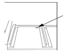
Vacuum or pressurized air applied to the outlet end of the drain tube must exist at the collection tray drain hole.
