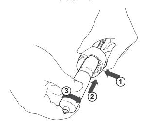
Figure 4: Align and push cartridge into the cap.
