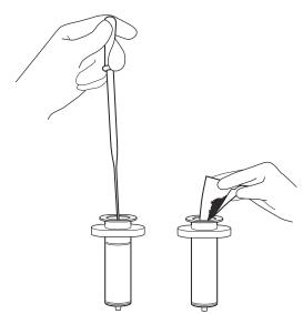
Figure 1: Preparing Cartridges Pipette sample onto prepacked cartridges (left) or pour adsorbed sample into empty cartridges (right).
