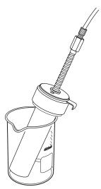
**Figure 6: Dry the sample** using the internal air pump on the Combi*Flash* Rf system (Optional)
