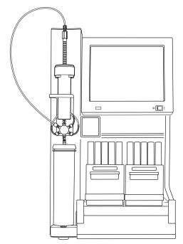
**Figure 5: Secure the cartridge assembly** on the system. (Combi*Flash* Rf 200 system shown.)
