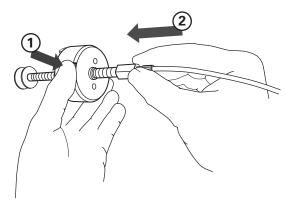
Figure 2: Press the lever and extend the plunger
