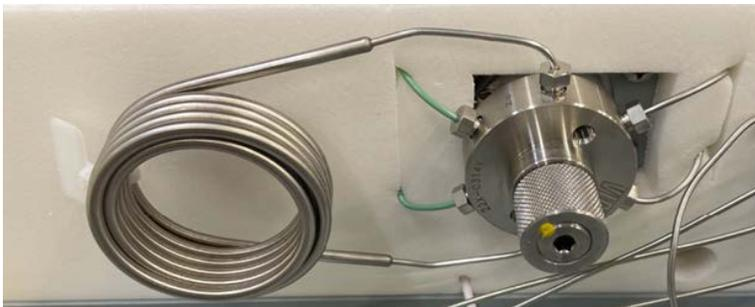
Figure 2-6 The sample injection valve
