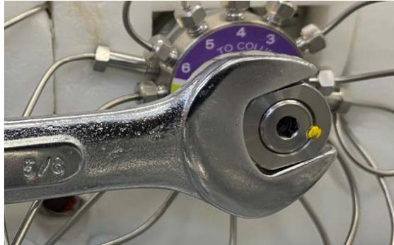
Figure 5-6 Loosening the rotor cap
