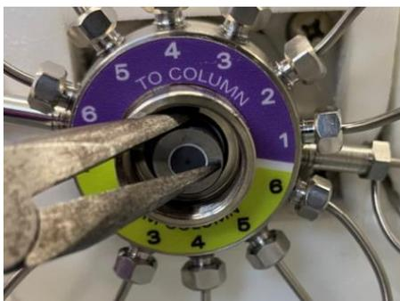
Figure 5-9 Tightening the new rotor
