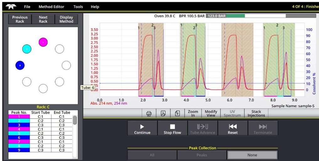
Figure 3-17 Four Stacked Injections with Time Windows Adjusted
