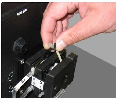
*Figure 5-22 Removing the tubing*
