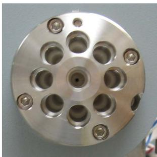
Figure 5-10 The fractionation valve
