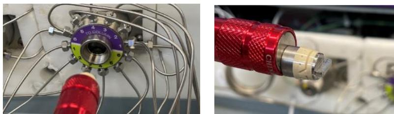
Figure 5-8 Removing the rotor
