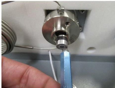
6. Make note of marking on rotor, as it needs to go back in the same orientation.
