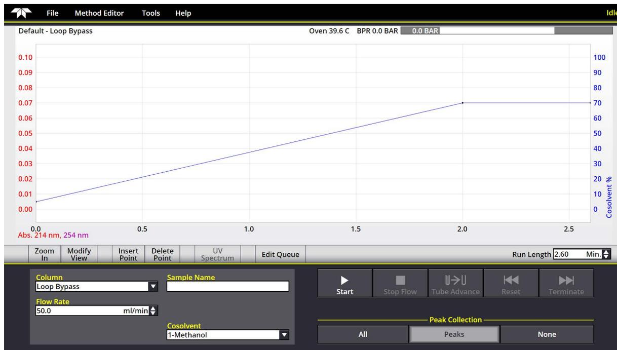
Figure 4-6 The Gradient Plot area
