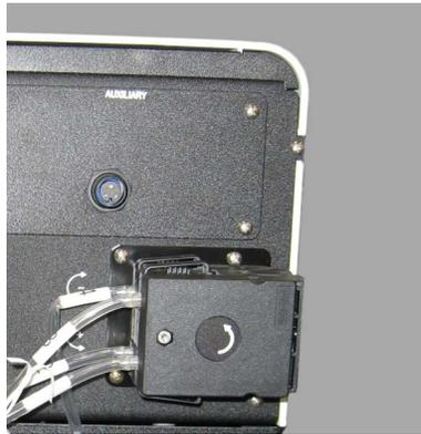
Figure 5-19 The peristaltic pump at the back of the AutoSampler
