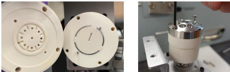
Figure 5-17 Reinstallation of the fractionation valve stator
