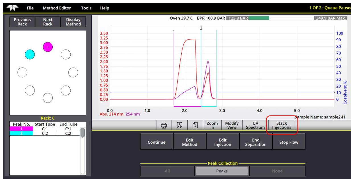
Figure 3-12 Higher sample loading, ready for stacked injections
