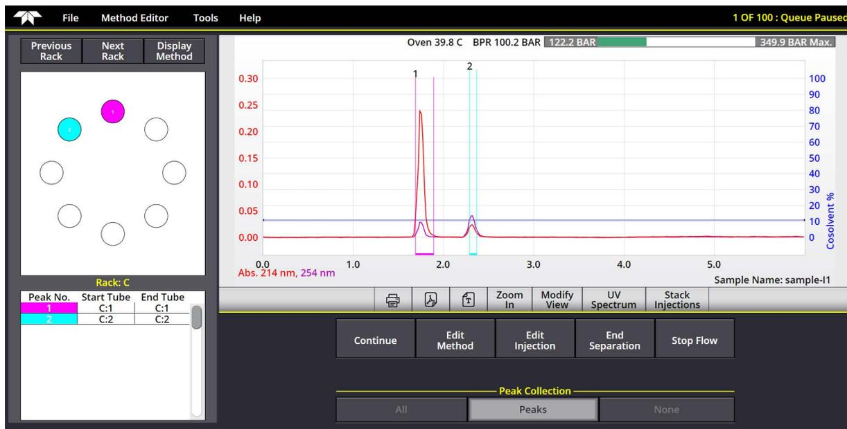
Figure 3-10 Chromatograph Showing High Resolution at End of Run
