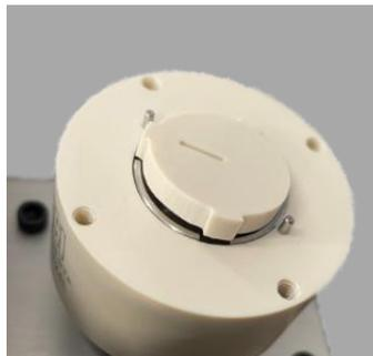
*Figure 5-15 Removal of the fractionation valve rotor*
