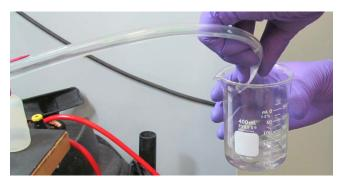
Figure 5-32 Draining the acetone into a 100 mL heaker
