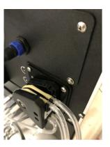
Figure 5-28 Attaching the new tubing
