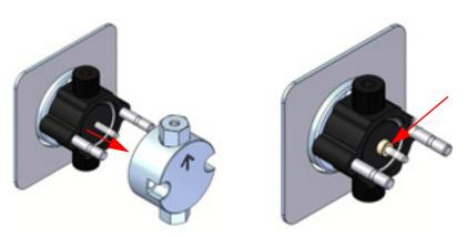
Figure 5-10 Removing the pump head
