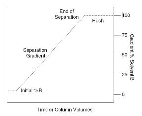
Figure 5-2 Default post-separation column and flow cell flush
