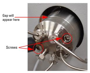
Figure 5-5 Location of screws on the stator retainer
