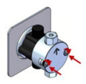
Figure 5-17 Reinstalling the fasteners
