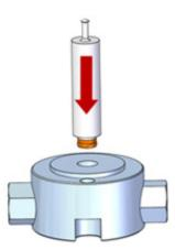
$Figure \ 5\text{-}14 Replacing \ the \ seal$
