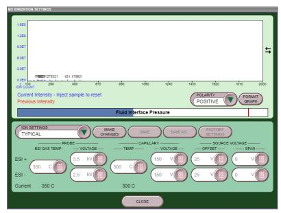
Figure 4-10 Mass Spectrometer Ionization Settings screen
