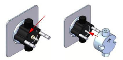
Figure 5-16 Reinstalling the pump head
