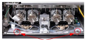
Pump assembly mounting screws
