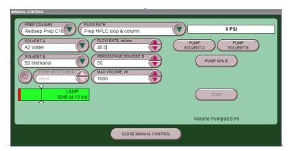
Figure 5-4 Manual Control Settings - Quick Cleaning-
