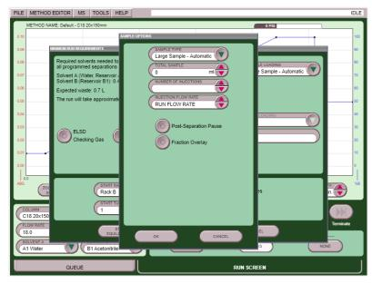
Figure 3-5 Dilute Sample Loading Pump Automatic Loading Screen
