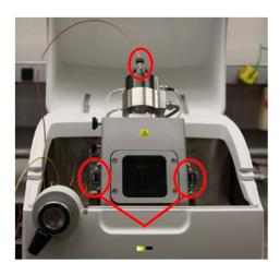
Figure 5-33 ESI and APCI removal from PurIon S and PurIon L
