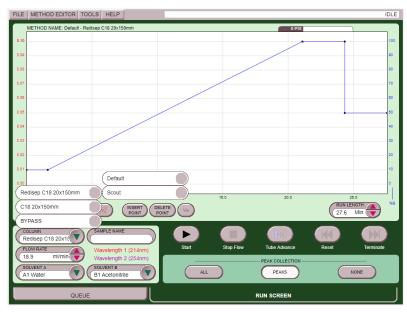
Figure 2-5 Loading the Scouting method
