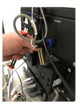
Figure 5-27 Removing the tubing
