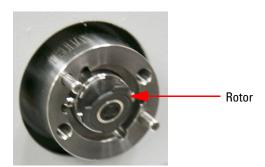
Figure 5-6 Removing the rotor
