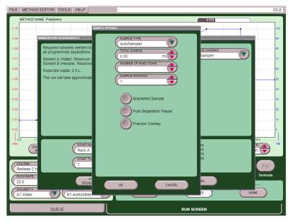
Figure 3-2 Selecting the sample volume and number of injections
