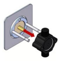
Figure 5-11 Removing the pump spacer block
