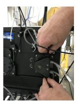
Figure 5-26 Removing the outer band
