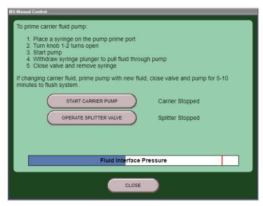
Figure 4-9 Mass Spectrometer Manual Control screen
