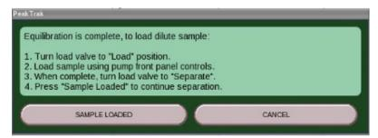
Figure 3-6 Loading Pump Manual screen
