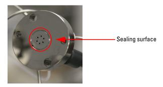
Figure 5-7 Sealing surface of the stator
