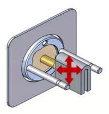
Figure 5-13 Cleaning the piston
