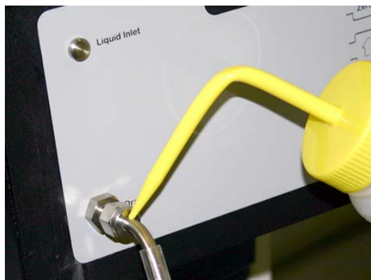
Figure 1-8 Attach drain adaptor; prime with mobile phase if desired
