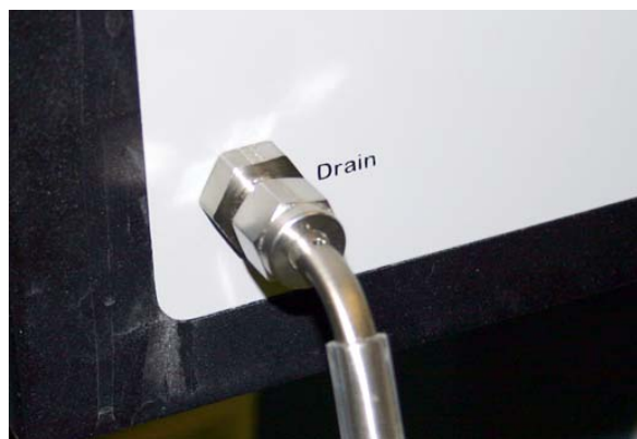
Figure 1-8 Attach drain adaptor; prime with mobile phase if desired
