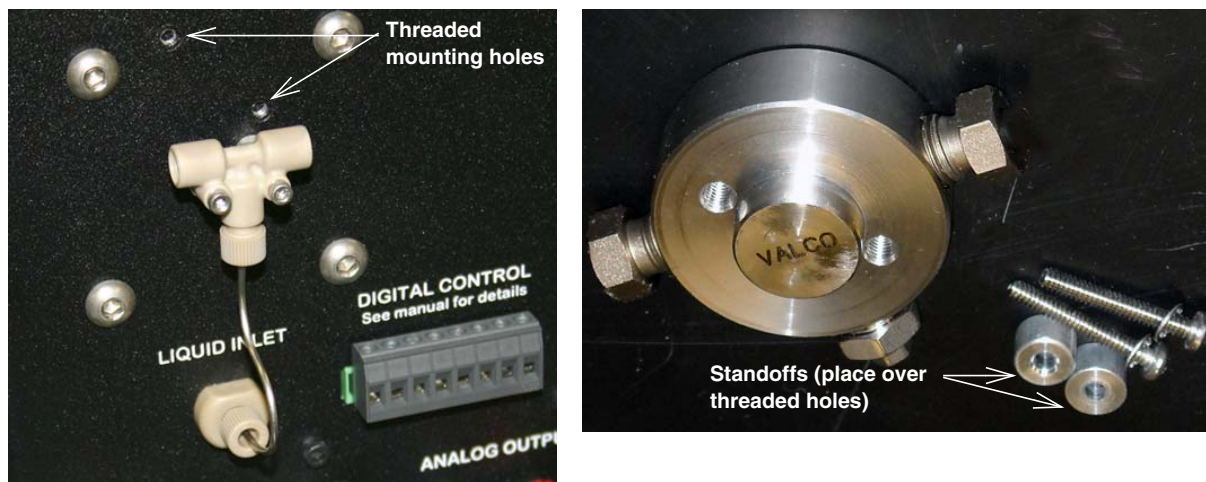
Figure 1-5 Replace the PEEK tee with the metal tee fitting
