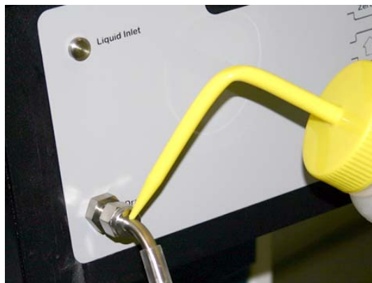
Figure 3-1 Attach drain adaptor; prime with mobile phase if desired
