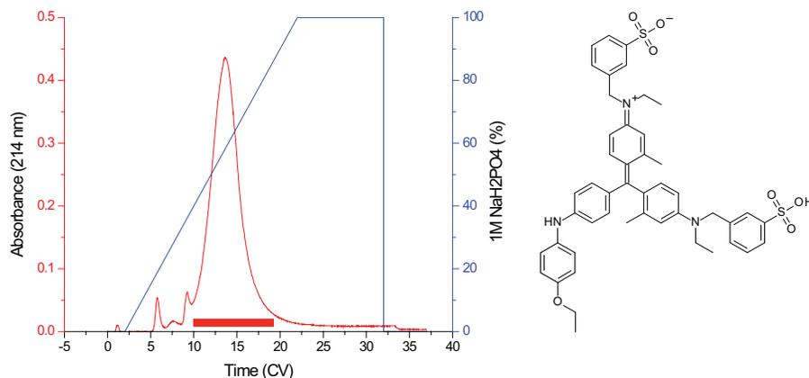
Figure 1: Purification of brilliant blue dye with a RediSep Rf Gold Column in WAX mode
