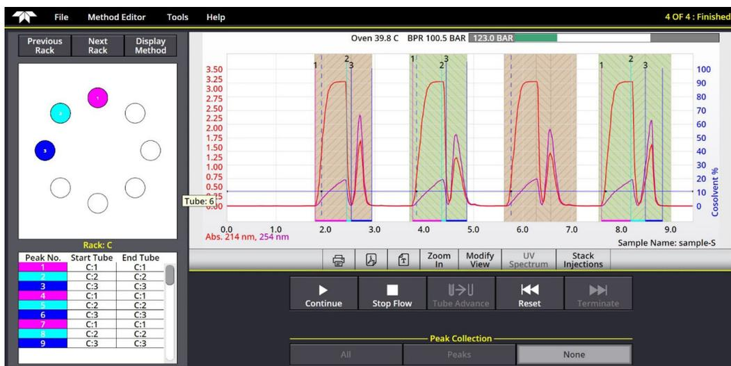
Figure 9. Four stacked injections with time windows adjusted during the run.
