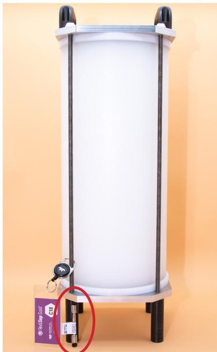
Figure 1. UHPLC column (circled) and an 8.6 kg C18 column
