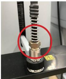
3. Connect the tube connected to the Torrent and the now free nut and ferrule and connect to the Union attached to the pre-swaged tubing.
