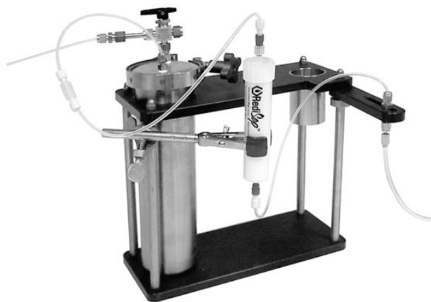
Figure 1: RediSep column on pressurized solvent reservoir system
