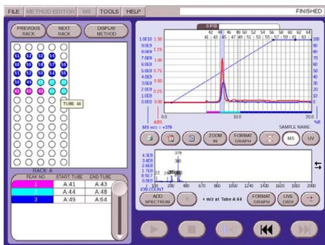
**Figure 4: Fraction Tube Composite Mass Spectrum is seen by selecting a tube on the touchscreen (tube 44 in this example)**
