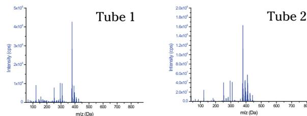
Figure 3: Purification of crude ergosterol with mass spectrometer and UV detection. Mass spectra show the contents of each collection fraction are the same.
