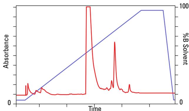
**Figure 3: Waters DeltaPrep 4000 system purification of 10 mg sample** of Compound A using a Vydac 10x250 mm column, 5 $\mu$  particle size
