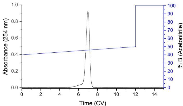
**Figure 2**–Benzophenone run on a RediSep Gold C8 column, 50 g, run with the same gradient used for Figure 1
