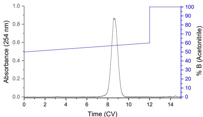
**Figure 4**–Benzophenone run on a RediSep Gold C18 column, 50 g, run with the same gradient used for Figure 3, in column volumes.
